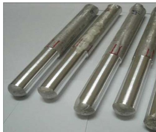
**Fig. 2** Test samples of AZ series Mg alloys
