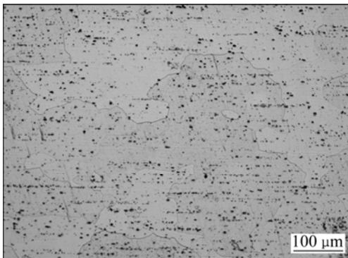
Fig. 4 Microstructures of Alloy 1 after hot working at (465 °C, 2 h) + (120 °C, 12 h)
