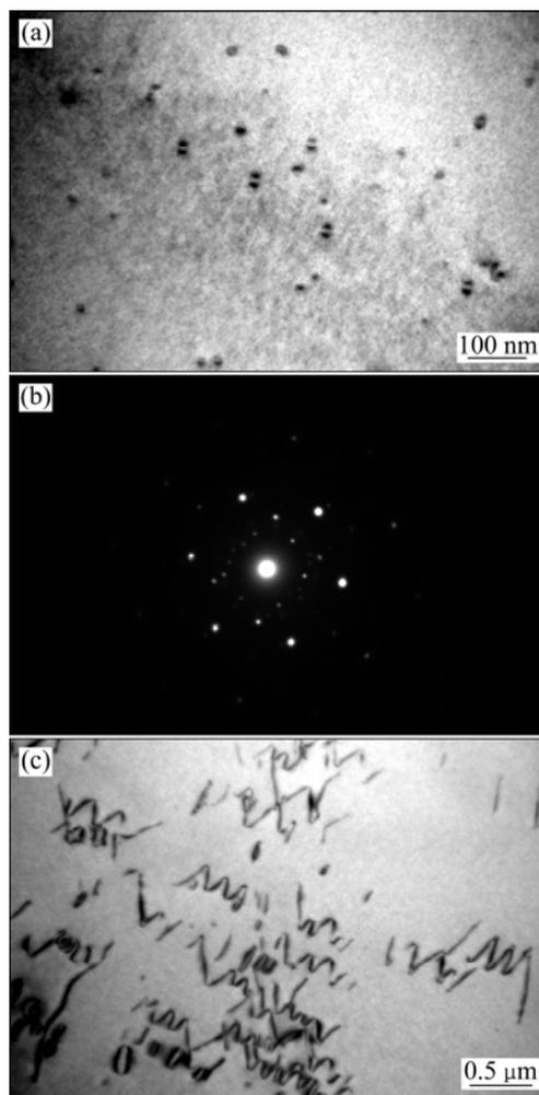
**Fig. 2** TEM images of Alloy 2: (a) Bright field image; (b) SAED pattern with  $[111]\text{Al}$  zone axis; (c) Pinning of the second phase grain on dislocation
