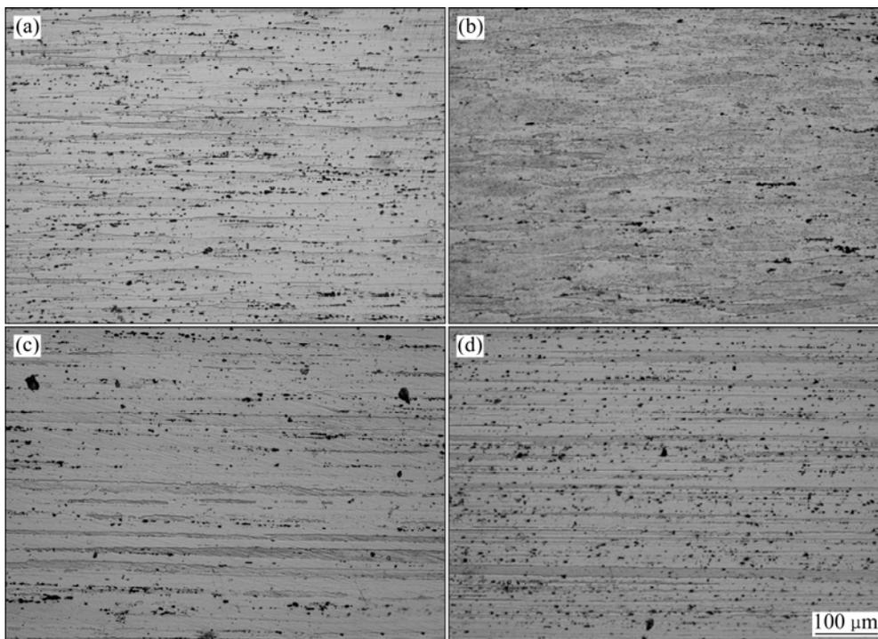
**Fig. 7** Microstructures of Alloy 2 after hot working at different conditions: (a) (420 °C, 6 h) + (465 °C, 2 h) + (120 °C, 12 h); (b) (420 °C, 3 h) + (465 °C, 3 h) + (120 °C, 12 h); (c) (420 °C, 3 h) + (465 °C, 2 h) + (120 °C, 12 h); (d) (200 °C, 3 h) + (420 °C, 3 h) + 465 °C, 2 h) + (120 °C, 12 h)
