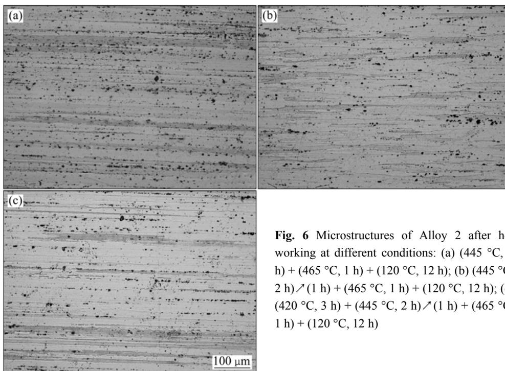
**Fig. 6** Microstructures of Alloy 2 after hot working at different conditions: (a) (445 °C, 2 h) + (465 °C, 1 h) + (120 °C, 12 h); (b) (445 °C, 2 h) / (1 h) + (465 °C, 1 h) + (120 °C, 12 h); (c) (420 °C, 3 h) + (445 °C, 2 h) / (1 h) + (465 °C, 1 h) + (120 °C, 12 h)
