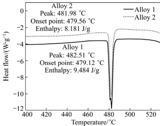
Fig. 3 DSC curves of two kinds of as-extruded alloys
