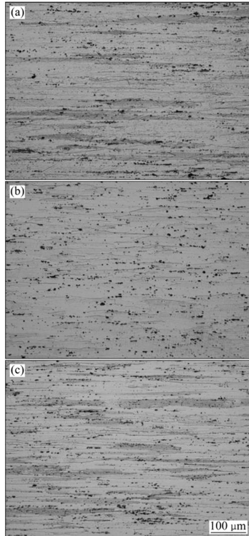
Fig. 5 Microstructures of Alloy 2 after hot working at different conditions: (a) (465 °C, 1 h) + (120 °C, 12 h); (b) (465 °C, 2 h) + (120 °C, 12 h); (c) (465 °C, 3 h) + (120 °C, 12 h)
