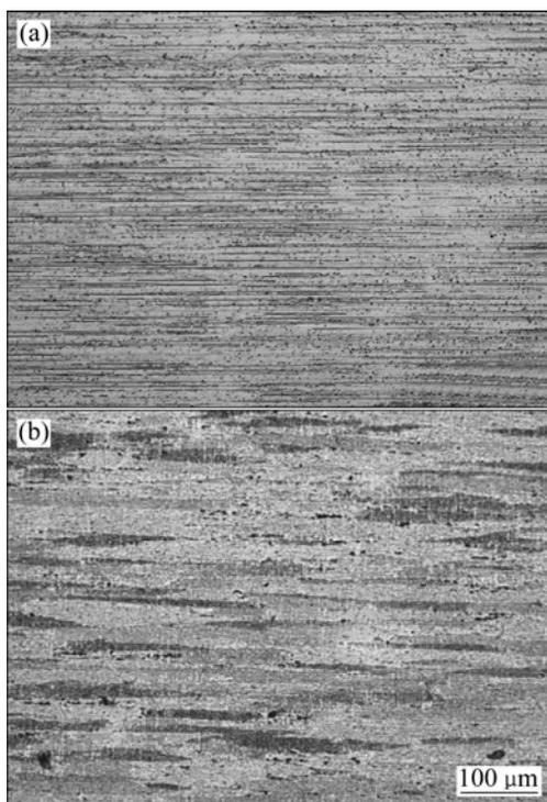
**Fig. 1** Microstructures of extruded alloy bars along longitudinal direction: (a) Alloy 1; (b) Alloy 2
