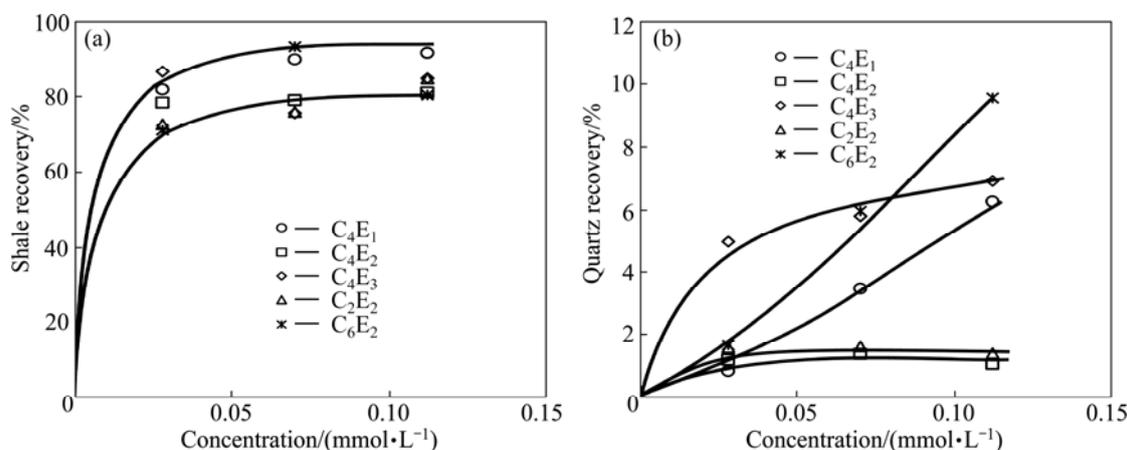
Fig. 2 Influence of ether concentration on recovery of shale (a) and quartz (b)
