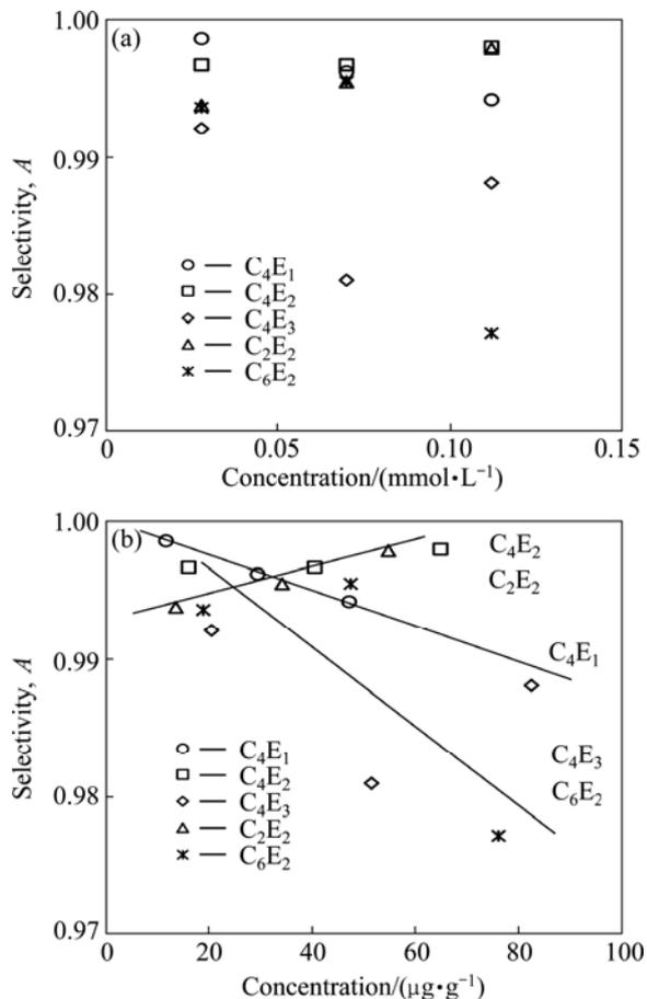
**Fig. 4** Influence of ether concentration on selectivity of carbonaceous copper shale and quartz mixture expressed in mmol/L (a) and  $\mu\text{g/g}$  (b)
