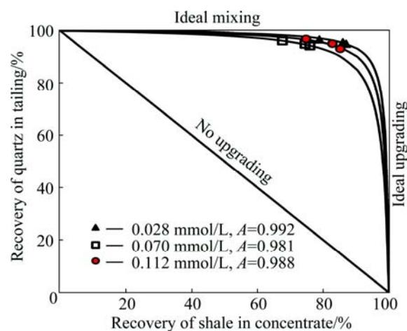
Fig. 3 Recovery of quartz in tailing versus recovery of carbonaceous copper shale in concentrate
