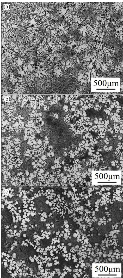
**Fig. 3** Optical microstructures of AZ91D semi-solid slurry prepared by gas bubbling under different gas flow rates: (a) 0; (b) 2 L/min; (c) 5 L/min
