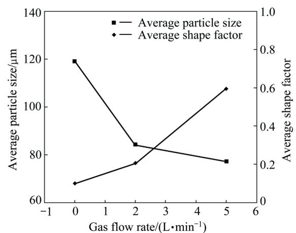
**Fig. 4** Effect of gas flow rate on average size and shape factor of primary  $\alpha$ -Mg particles in AZ91D semi-solid slurry
