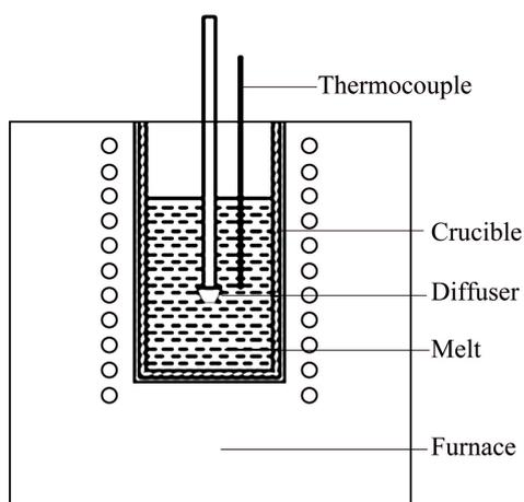
Fig. 1 Schematic of equipment used for gas bubbling
