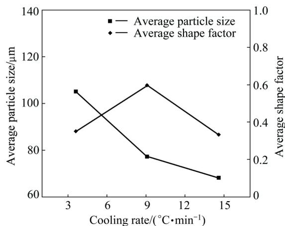
**Fig. 6** Effect of cooling rate on average size and shape factor of primary  $\alpha$ -Mg particles in AZ91D semi-solid slurry
