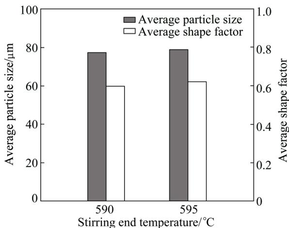
**Fig. 8** Effect of stirring end temperature on average size and shape factor of primary  $\alpha$ -Mg particles in AZ91D semi-solid slurry
