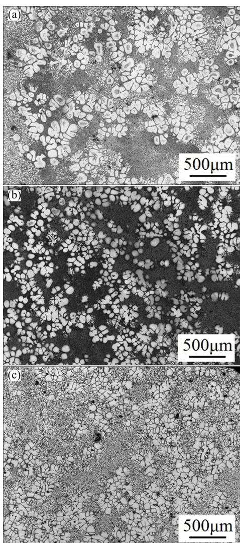
**Fig. 5** Optical microstructures of AZ91D alloy slurry prepared by gas bubbling under different cooling rates: (a) 3.6 °C/min; (b) 9.1 °C/min; (c) 14.6 °C/min
