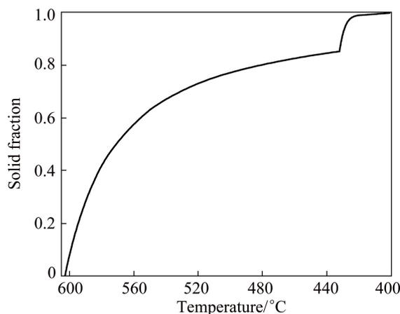
Fig. 2 Curve of solid fraction versus temperature of AZ91D alloy based on Scheil equation
