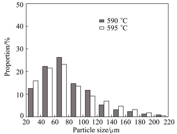
**Fig. 9** Effect of stirring end temperature on size distribution of primary  $\alpha$ -Mg particles in AZ91D semi-solid slurry
