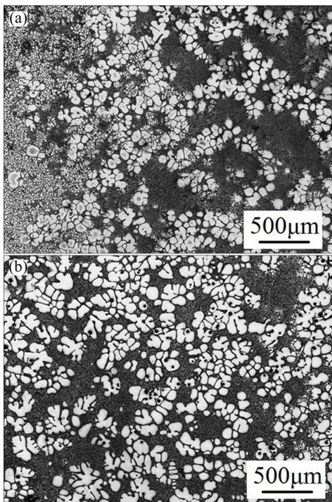
**Fig. 7** Optical microstructures of AZ91D semi-solid slurry prepared by gas bubbling with different stirring end temperatures: (a) 590 °C; (b) 595 °C
