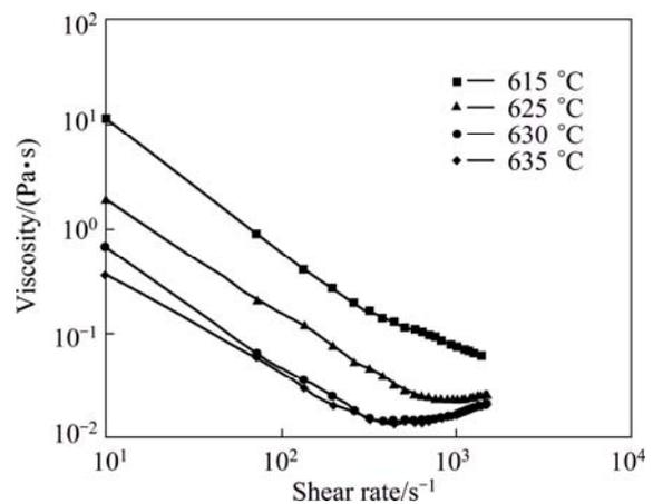
Fig. 5 Variation of viscosity with shear rate at different temperatures
