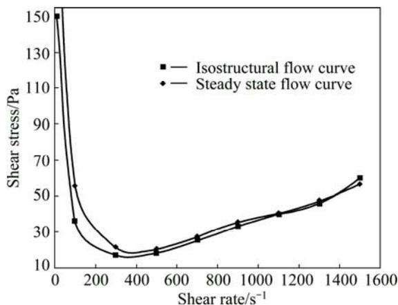
Fig. 8 Isostructural and steady state flow curves
