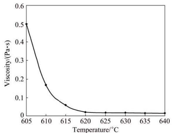
Fig. 4 Variation of viscosity with temperature at fixed shear rate of  $700 \text{ s}^{-1}$
