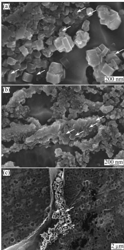
**Fig. 6** Distribution of non-deformable  $\text{TiB}_2$  particles (hexagonal in shape marked by arrows) deposited at two different locations along grain boundaries in semi-solid processed sample (a, b) and in as-cast sample (c)
