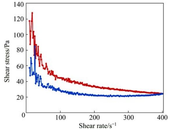
Fig. 9 Hysteresis loops generated during thixotropic tests
