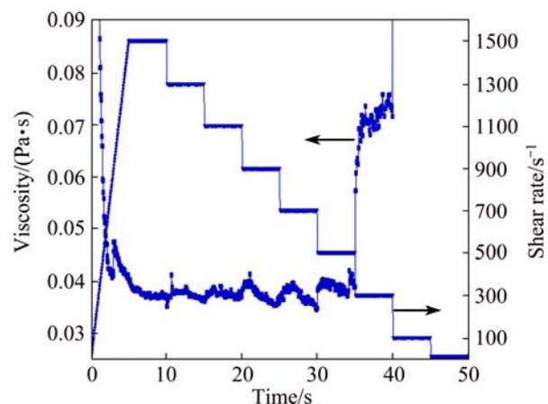
**Fig. 7** Variation of viscosity with time jumps in shear rate
