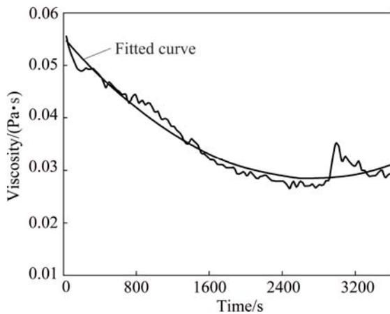
Fig. 3 Variation of viscosity with time at fixed shear rate of  $600 \text{ s}^{-1}$
