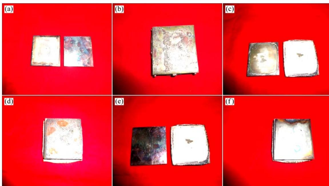
**Fig. 1** Fabricated diffusion bonded coupons: (a) Bonding temperature lower than 700 °C; (b) Bonding temperature higher than 825 °C; (c) Bonding pressure lower than 2 MPa; (d) Bonding pressure higher than 5 MPa; (e) Bonding time less than 15 min; (f) Bonding time longer than 120 min
