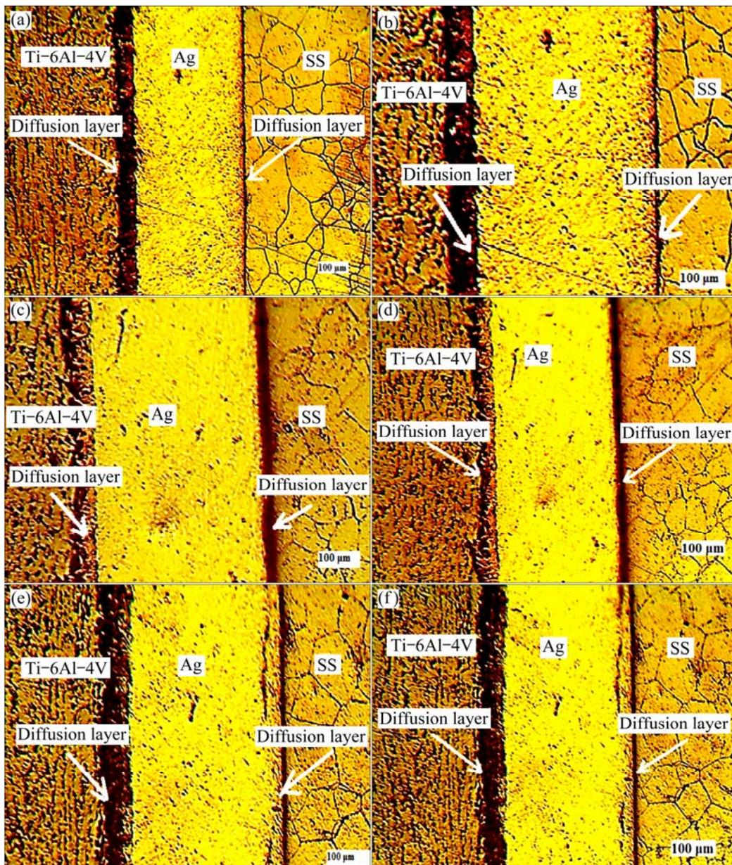
**Fig. 4** Optical micrographs of joint bonded under different conditions: (a) Joint No.15; (b) Joint No. 19; (c) Joint No.18; (d) Joint No. 34; (e) Joint No. 31; (f) Joint No. 24
