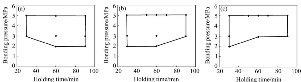
Fig. 3 Pressure–time diagrams of DBW at different temperatures: (a) 700 °C; (b) 750 °C; (c) 800 °C
