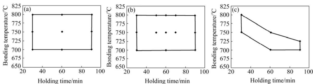
Fig. 2 DBW of titanium alloy stainless steel under different pressures: (a) 3 MPa; (b) 5 MPa; (c) 2 MPa
