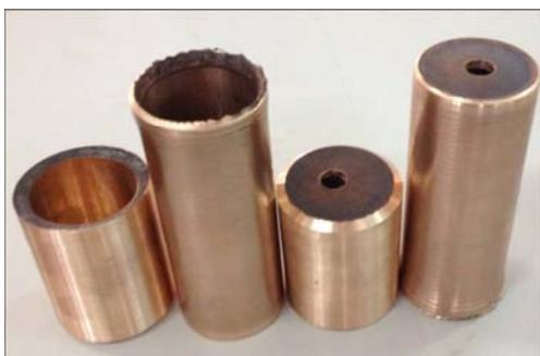
**Fig. 1** Tin–bronze connecting rod bushing parts before and after power spinning
