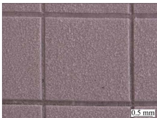
Fig. 5 Polarized light microscope image for MgAl-LDH coating treated for 8 h on aluminum alloy surface after adhesion test by ASTM standard D 3359–02 method B
