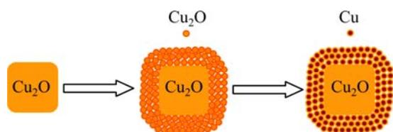
Fig. 6 Schematic diagram of  $\text{Cu}_2\text{O}@Cu_2\text{O}$  core-shell NP conversion to  $\text{Cu}_2\text{O}@Cu$  core-shell NP
