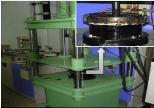
**Fig. 2** Experimental test rig with enlarged view of die with induction furnace
