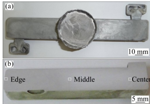
Fig. 3 AA7075 alloy part produced by thixocasting (a) and metallographic examination regions of thixocast specimen (b)
