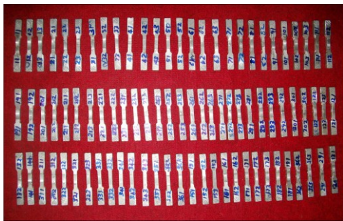
Fig. 7 Batch of prepared tensile specimens
