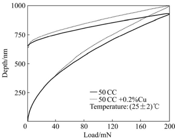
**Fig.8** Curves of representative load vs depth in nano-indentation tests
