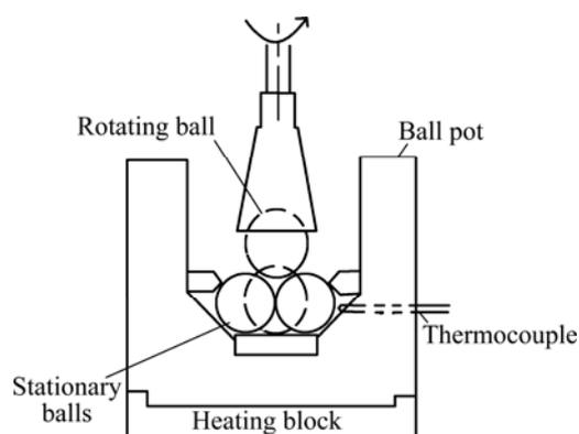
Fig.2 Schematic diagram of four-ball tester
