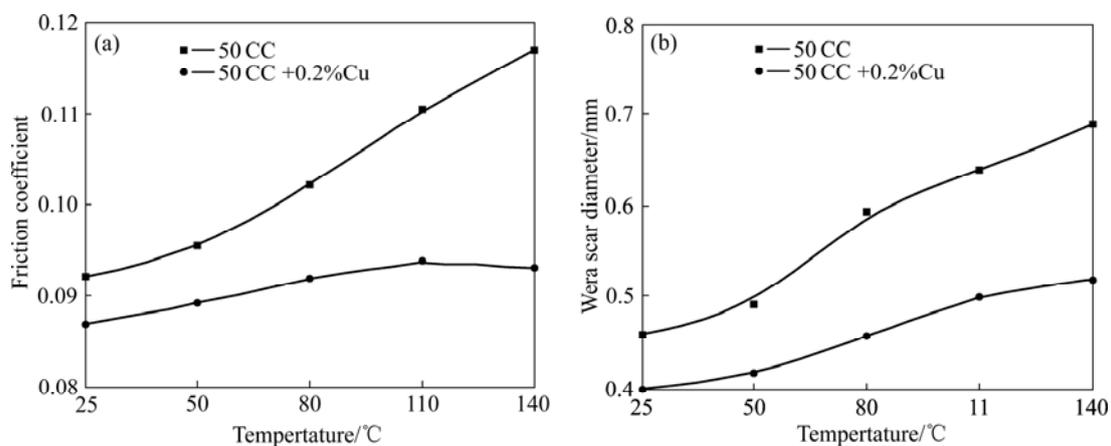
**Fig.3** Tribological properties as function of temperature: (a) Friction coefficient; (b) Wear scar diameter
