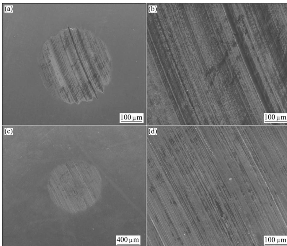
**Fig.4** Typical SEM images of worn surfaces lubricated with different oil at 140 °C: (a, b) 50CC; (c, d) 50CC+0.2%Cu
