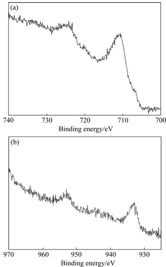
**Fig.7** XPS analysis of worn surface lubricated with 50CC oil+0.2% Cu: (a) Fe 2p; (b) Cu 2p
