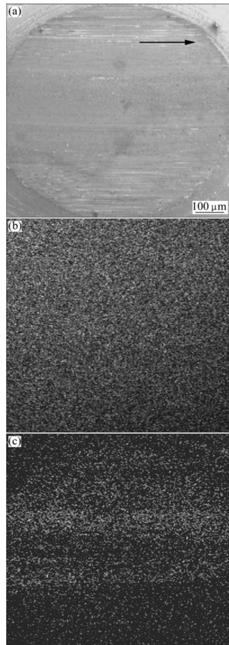
**Fig.6** EDS analysis of worn surface lubricated with 50CC oil+0.2%Cu: (a) Surface morphology; (b) Fe distribution map; (c) Cu distribution map (Arrow indicates friction direction)
