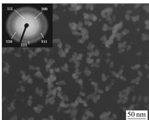
Fig.1 TEM image and ED pattern of Cu nanoparticles
