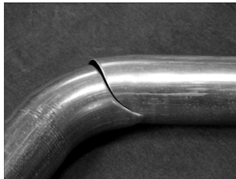
Fig.5 Tube crack shape at high bending velocity
