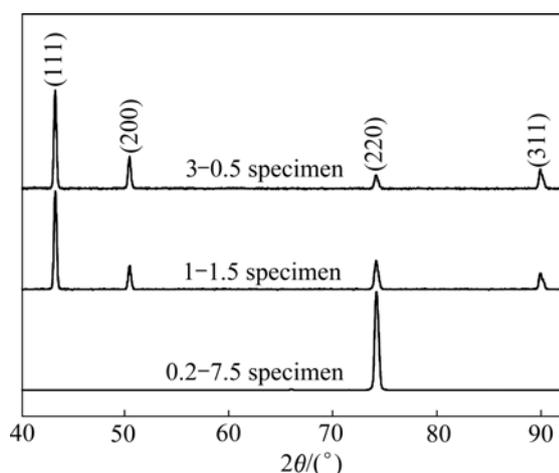
Fig.3 XRD patterns of FCCL specimens
