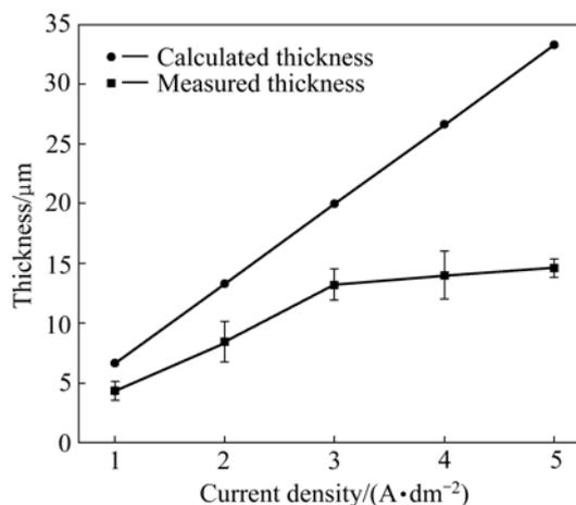
Fig.1 Variation in thickness of Cu layer with current density
