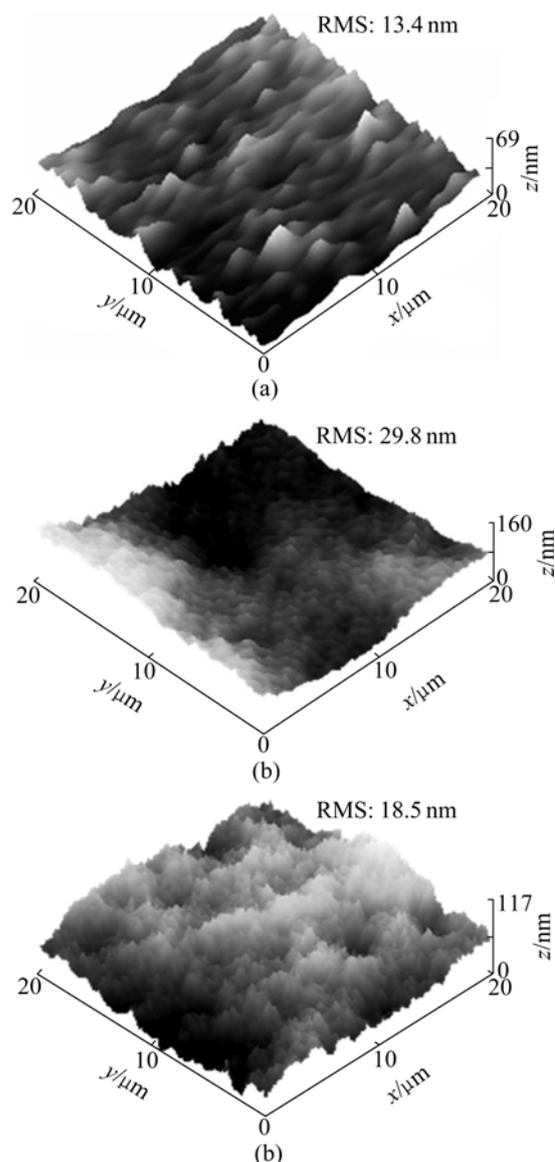
**Fig.2** AFM profiles (20  $\mu\text{m} \times 20 \mu\text{m}$ ) of surfaces: (a) Electroless-plated Cu/PI; (b) 1–1.5 specimen; (c) 3–0.5 specimen
