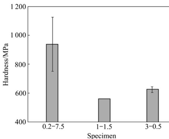
Fig.4 Dependence of hardness of Cu layer on current density
