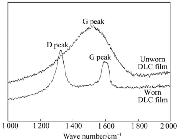
**Fig.4** Raman graph of worn and unworn ring specimens with DLC coatings
