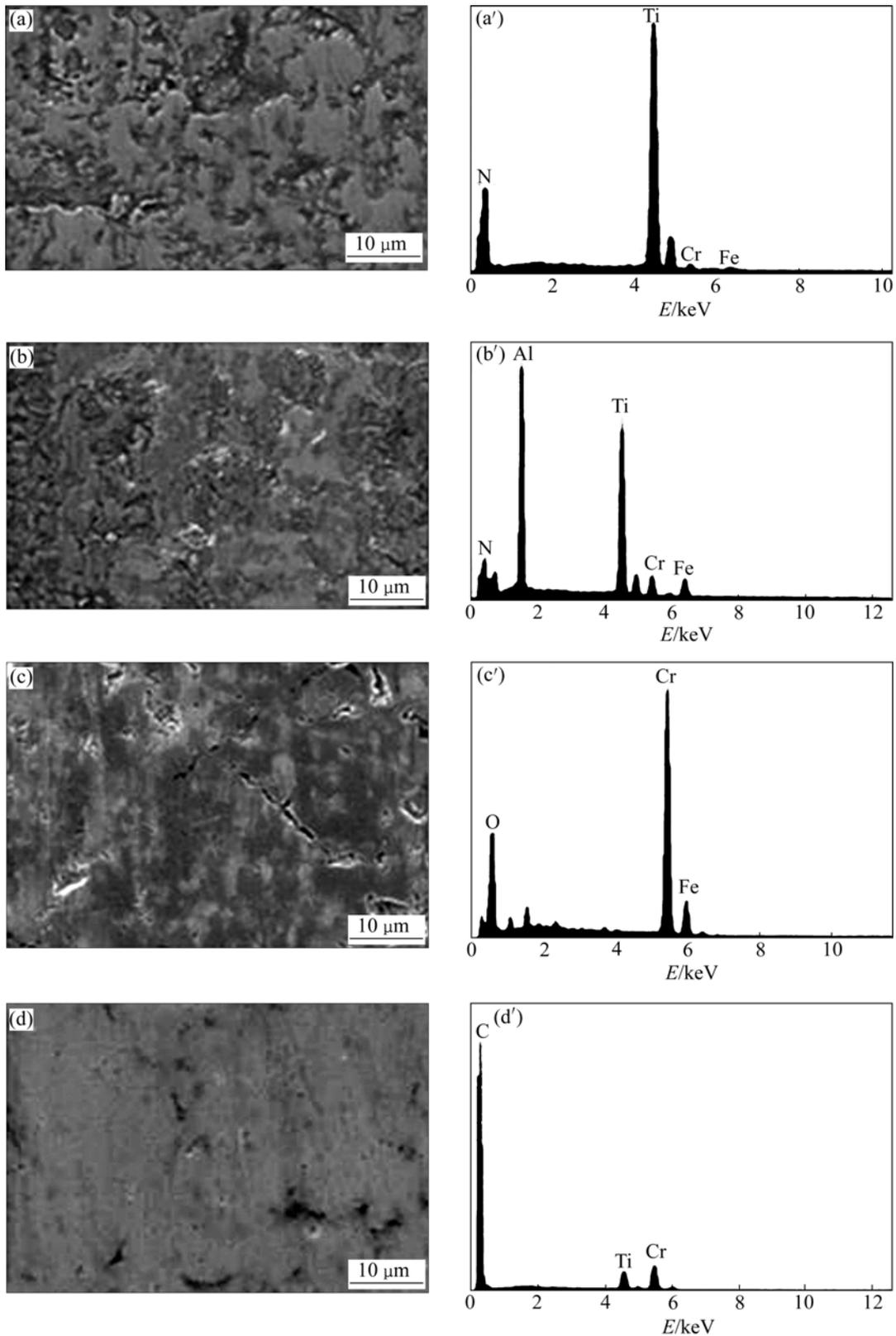
**Fig.3** SEM images and EDX spectra of worn ring specimens with coatings: (a), (a') TiN; (b), (b') TiAlN; (c), (c') Cr-ceramic; (d), (d') DLC
