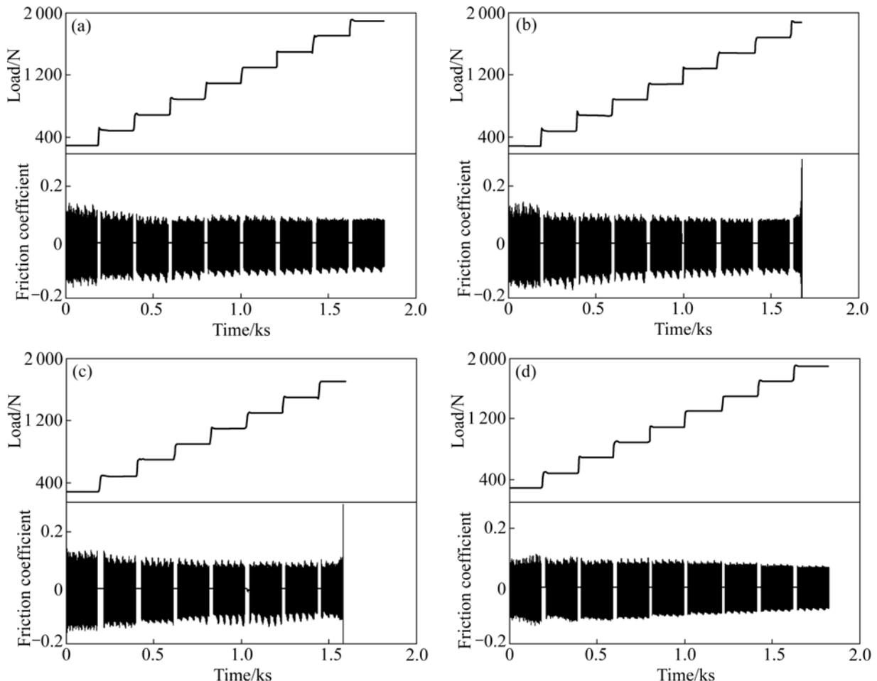
**Fig.5** Time to scuffing failures with different coated piston rings: (a) TiN coated piston ring; (b) TiAlN coated piston ring; (c) Cr-ceramic coated piston ring; (d) DLC coated piston ring
