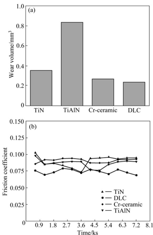
**Fig.2** Wear volumes (a) and friction coefficients (b) of cylinder blocks with different coatings
