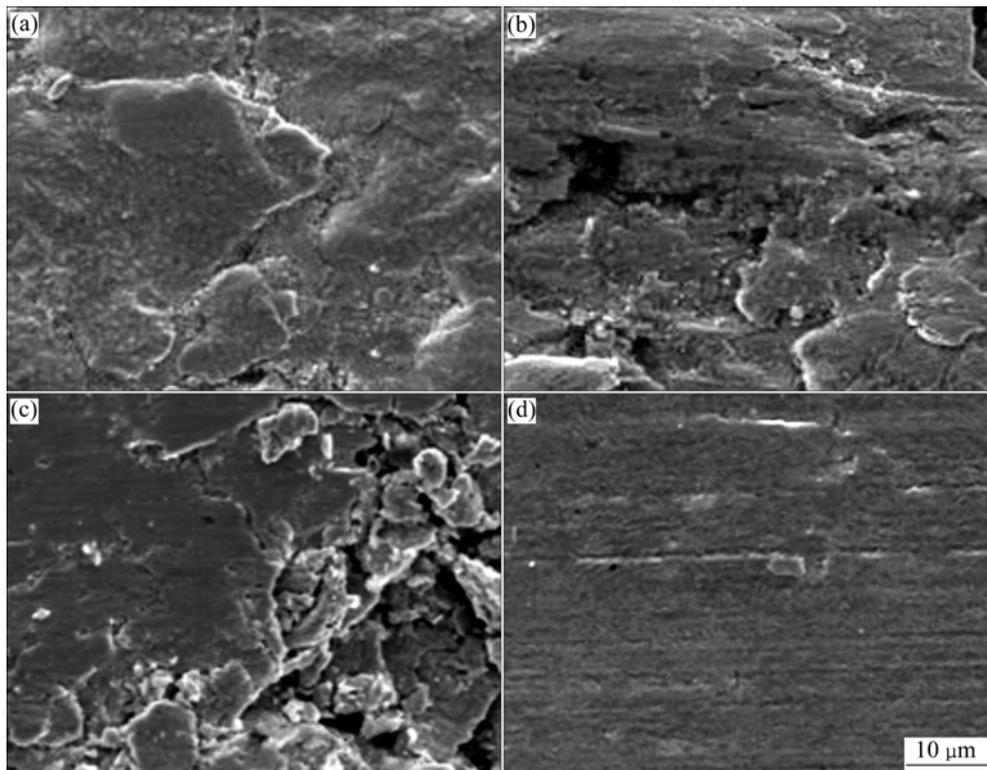
**Fig.6** SEM images of worn cylinder specimens after scuffing tests: (a) TiN coating; (b) TiAlN coating; (c) Cr-ceramic coating; (d) DLC coating
