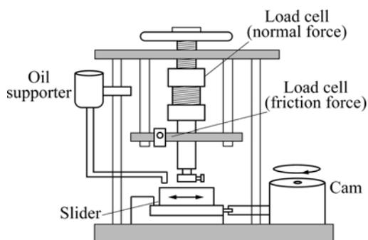
**Fig.1** Schematic drawing of reciprocating wear tester
