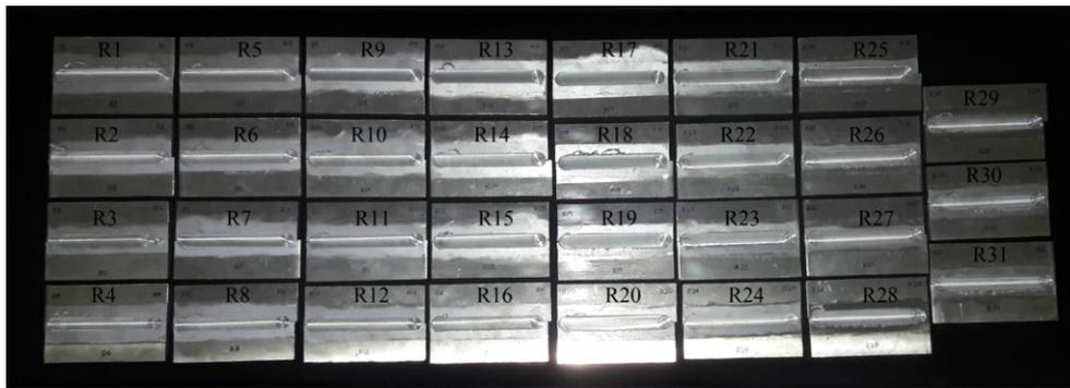
Fig. 2 Photographs of FS welded joints by different FSW parameter combinations
