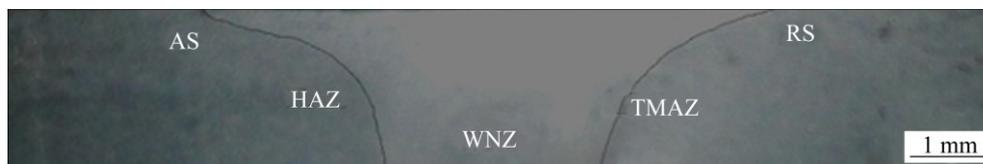
Fig. 5 Cross sectional macrograph of welded specimen with high tensile strength
