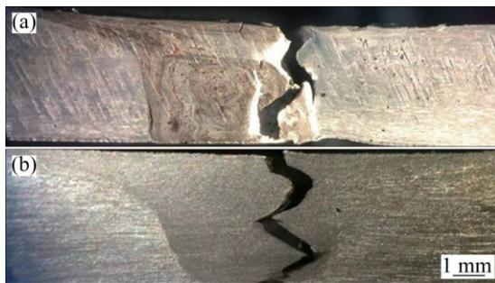
**Fig. 15** Fracture location of joints: (a) Al/Cu/Al; (b) Al/Al
