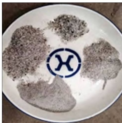
Fig. 1 CRT funnel glasses with different particle sizes
