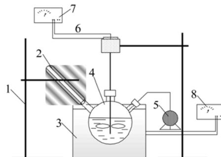
**Fig.1** Schematic diagram of experimental installation: 1 Fastening stand; 2 Condenser; 3 Thermostat water bath; 4 Flask reactor; 5 Feed dosing pump; 6 DC electromotor; 7 Voltage regulator; 8 Digital multimeter
