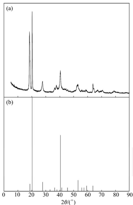
**Fig.4** XRD spectra of Bayerite standard and product prepared at optimum condition: (a) Product; (b) Bayerite standard
