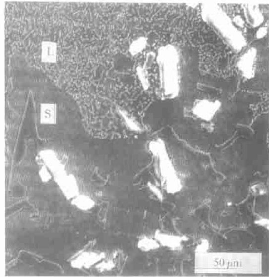
Fig. 3 Distribution of particles at solid/liquid interface in Al_2O_3p/ Al-Si-Sr-Ca composites ( R = 5.56 \times 10^{-4} \text{ mm/s} )
