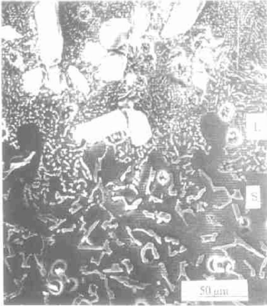
Fig.1 Distribution of particles at solid/liquid interface in Al_2O_3p/ Al-Si-Sr composites ( Upward solidification , R = 2.22 \times 10^{-3} \text{ mm/s.} )
