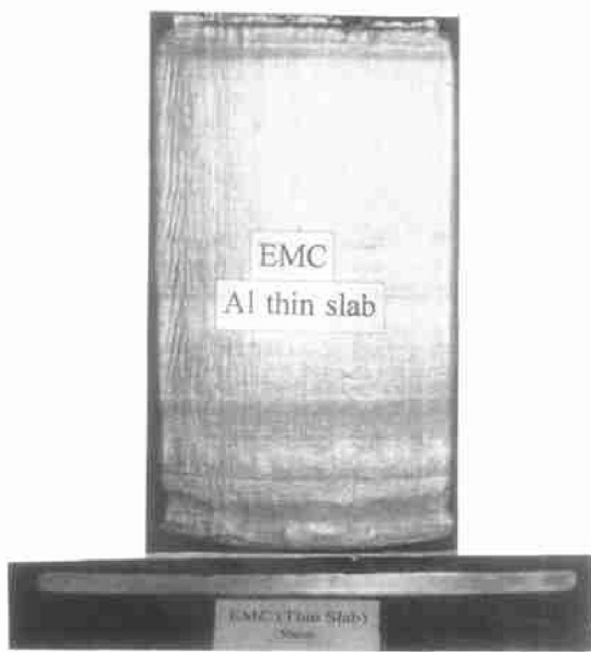
Fig.8 Sample of Al thin slab (480 mm × 20 mm × 850 mm)
