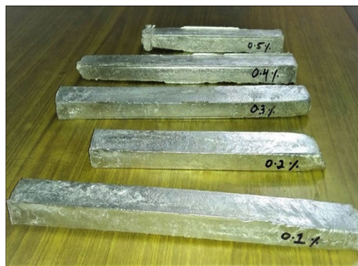
Fig. 1 Stir cast samples with varying amounts of yttrium addition
