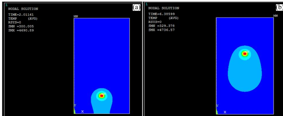
**Fig. 8** Temperature distribution for moving heat source at different time: (a) 2 s; (b) 6 s (current 110 mA, voltage 50 kV and weld speed 600 mm/min)
