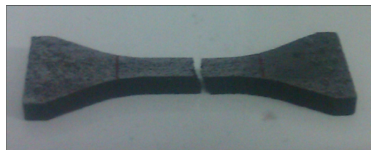
Fig. 5 Tensile fracture specimen of porous FeAl
