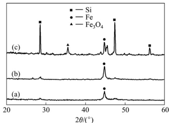
Fig.1 Influence of milling time on phase structure: (a) 50 h; (b) 38 h; (c) 20 h
