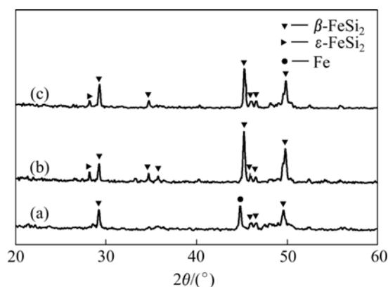
Fig.2 Influence of sintering conditions on phase structure: (a) 930 °C, 10 h; (b) 930 °C, 15 h; (c) 890 °C, 15 h
