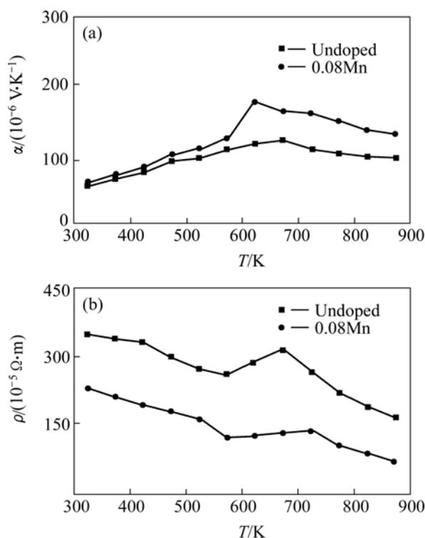
**Fig.3** Temperature dependence of thermoelectric and electrical parameters of  $\text{FeSi}_2$  and  $\text{Fe}_{0.92}\text{Mn}_{0.08}\text{Si}_2$ : (a) Seebeck coefficient; (b) Electrical resistivity
