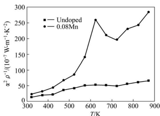
**Fig.4** Temperature dependence of power factor of  $\text{FeSi}_2$  and  $\text{Fe}_{0.92}\text{Mn}_{0.08}\text{Si}_2$
