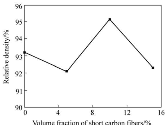
**Fig.1** Relative density of  $C_{sf}/Si_3N_4$  composites with different volume fractions of short carbon fibers
