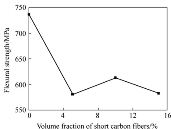
**Fig.3** Relationship between volume fraction of short carbon fibers and flexural strength of  $C_{sf}/Si_3N_4$  composites
