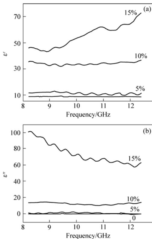
**Fig.4** Real part ( $\epsilon'$ ) and imaginary part ( $\epsilon''$ ) of permittivity of  $C_{sf}/Si_3N_4$  composites as function of frequency at different volume fractions of short carbon fibers
