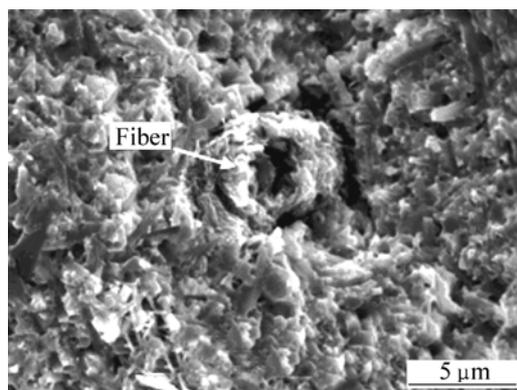
**Fig.2** Microphotograph of  $C_{sf}/Si_3N_4$  composites with 5% short carbon fibers
