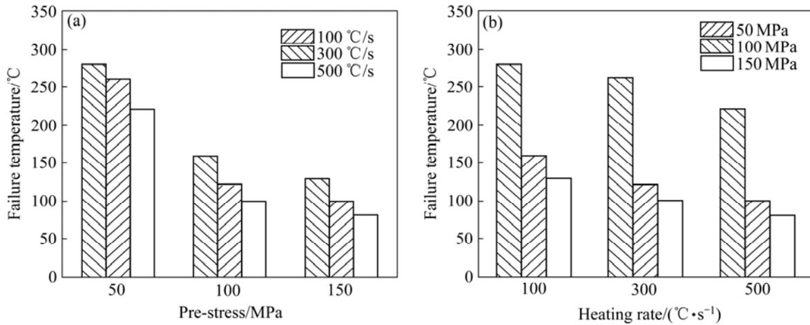
**Fig.4** Failure temperatures at different pre-stresses and heating-rates: (a) Failure temperature vs pre-stress; (b) Failure temperature vs heating rates
