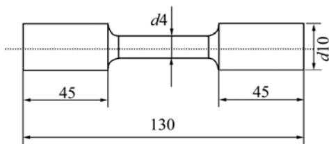
Fig.1 Draft of specimen (Unit: mm)
