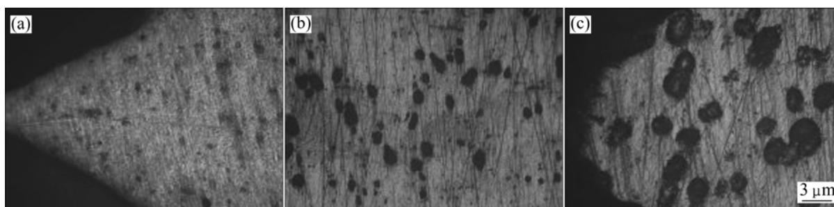
**Fig.7** Metallographs at pre-stress  $\sigma=150$  MPa and different heating rates: (a) 100 °C/s; (b) 300 °C/s; (c) 500 °C/s
