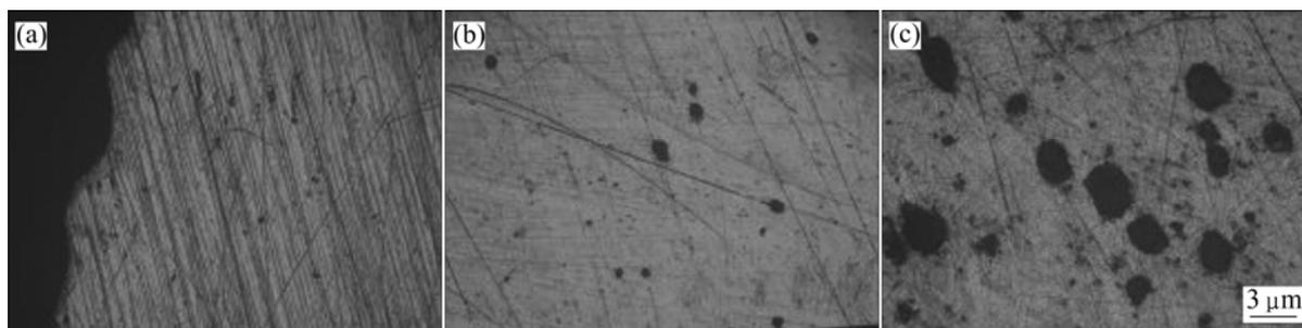
**Fig.5** Metallographs at pre-stress of  $\sigma=50$  MPa and different heating rates: (a) 100 °C/s; (b) 300 °C/s; (c) 500 °C/s
