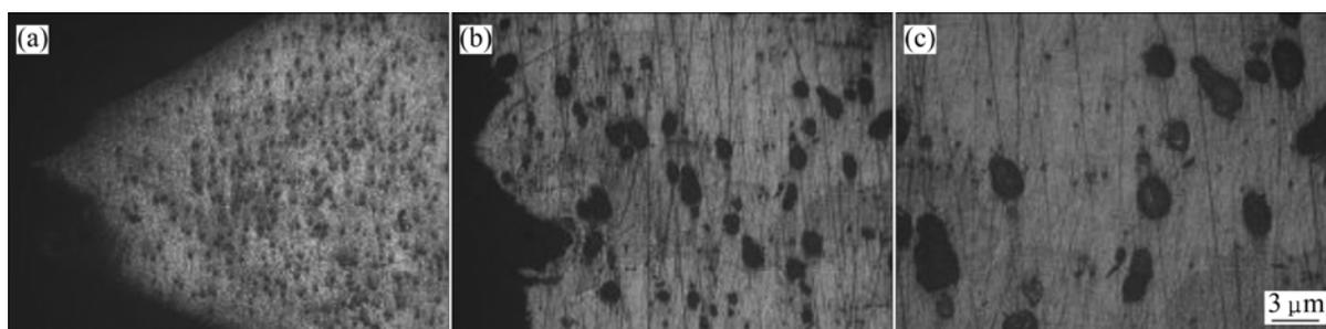
**Fig.6** Metallographs at pre-stress  $\sigma=100$  MPa and different heating rates: (a) 100 °C/s; (b) 300 °C/s; (c) 500 °C/s
