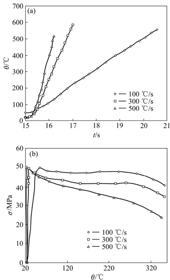
Fig.2 Testing results at different heating rates with  $\sigma=50$  MPa: (a) Temperature vs time; (b) Stress vs temperature
