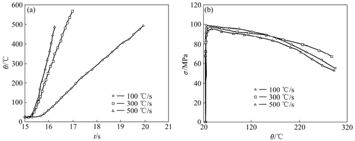
**Fig.3** Testing results at different heating rates with  $\sigma=100$  MPa: (a) Temperature vs time; (b) Stress vs temperature
