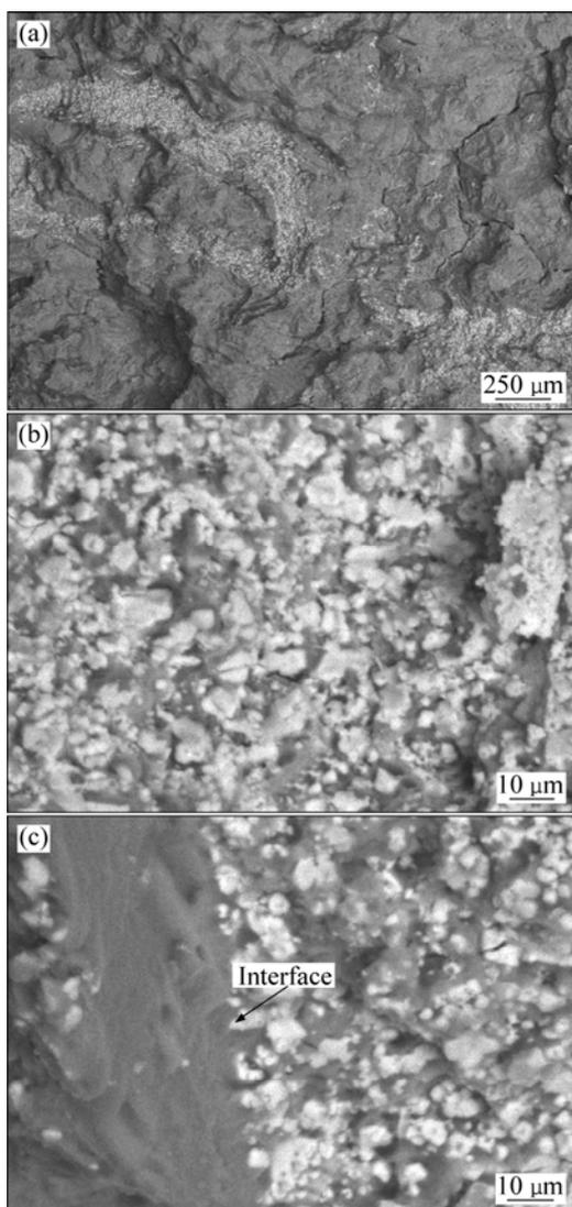
**Fig.4** SEM images of fracture surface of interpenetrating composites: (a) Overview; (b) Strut at high magnification; (c) Interface between struts and matrix
