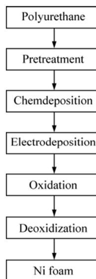
**Fig.1** Preparation process of nickel foam reinforcement
