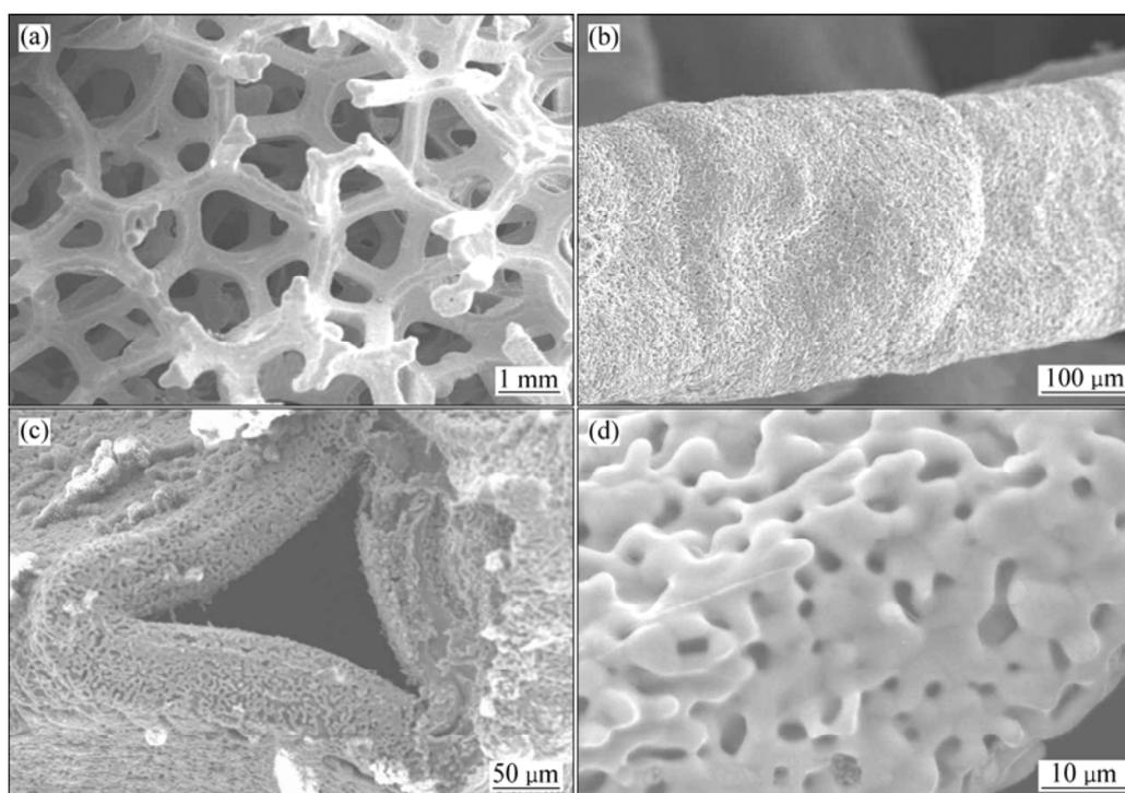
**Fig.2** Morphologies of Ni foam reinforcement: (a) Foam, in low magnification; (b) Strut, in low magnification; (c) Cross section of strut; (d) Surface of strut
