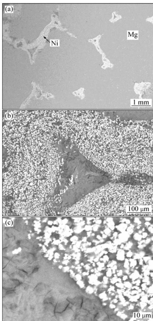
**Fig.3** Morphologies of Ni foam/Mg interpenetrating composites: (a) Low magnification image; (b) Higher magnification image; (c) Interface
