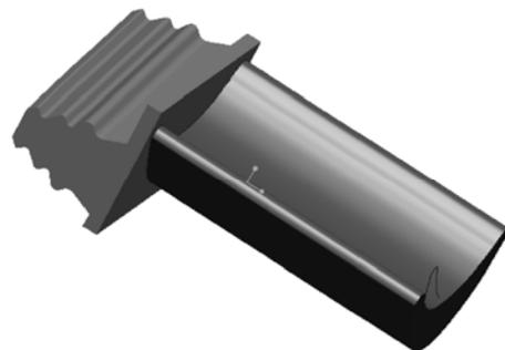
Fig.1 Blade of air-turbine
