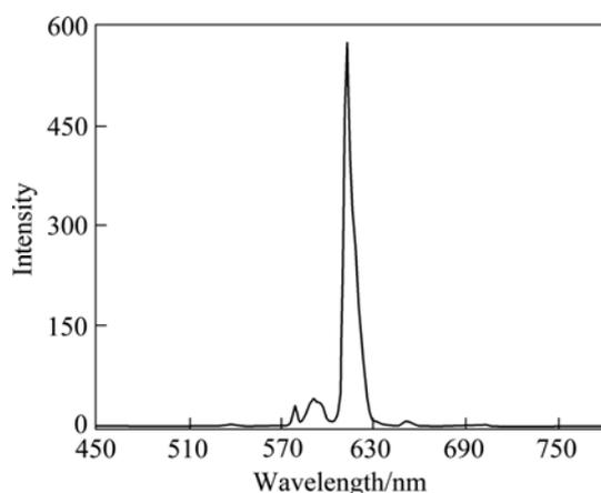
**Fig.4** Typical emission spectrum of complex  $\text{Eu}(\text{TТА})_3(2\text{NH}_2\text{-Phen})$  excited at 332 nm
