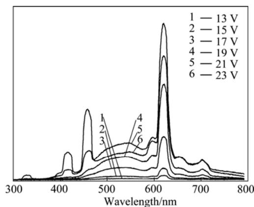
**Fig.5** EL spectra of complex  $\text{Eu}(\text{TТА})_3(2\text{NH}_2\text{-Phen})$  at various driving voltages
