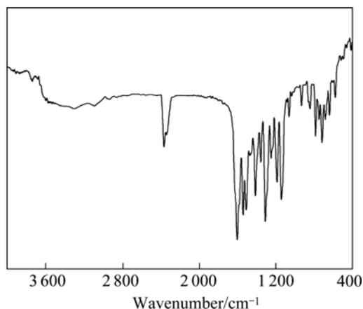
Fig.1 Infrared spectrum of complex  $\text{Eu}(\text{TТА})_3(2\text{NH}_2\text{-Phen})$
