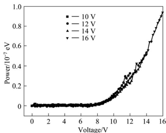
**Fig.6** Power — voltage curves for complex  $\text{Eu}(\text{TТА})_3(2\text{NH}_2\text{-Phen})$  at various driving voltages
