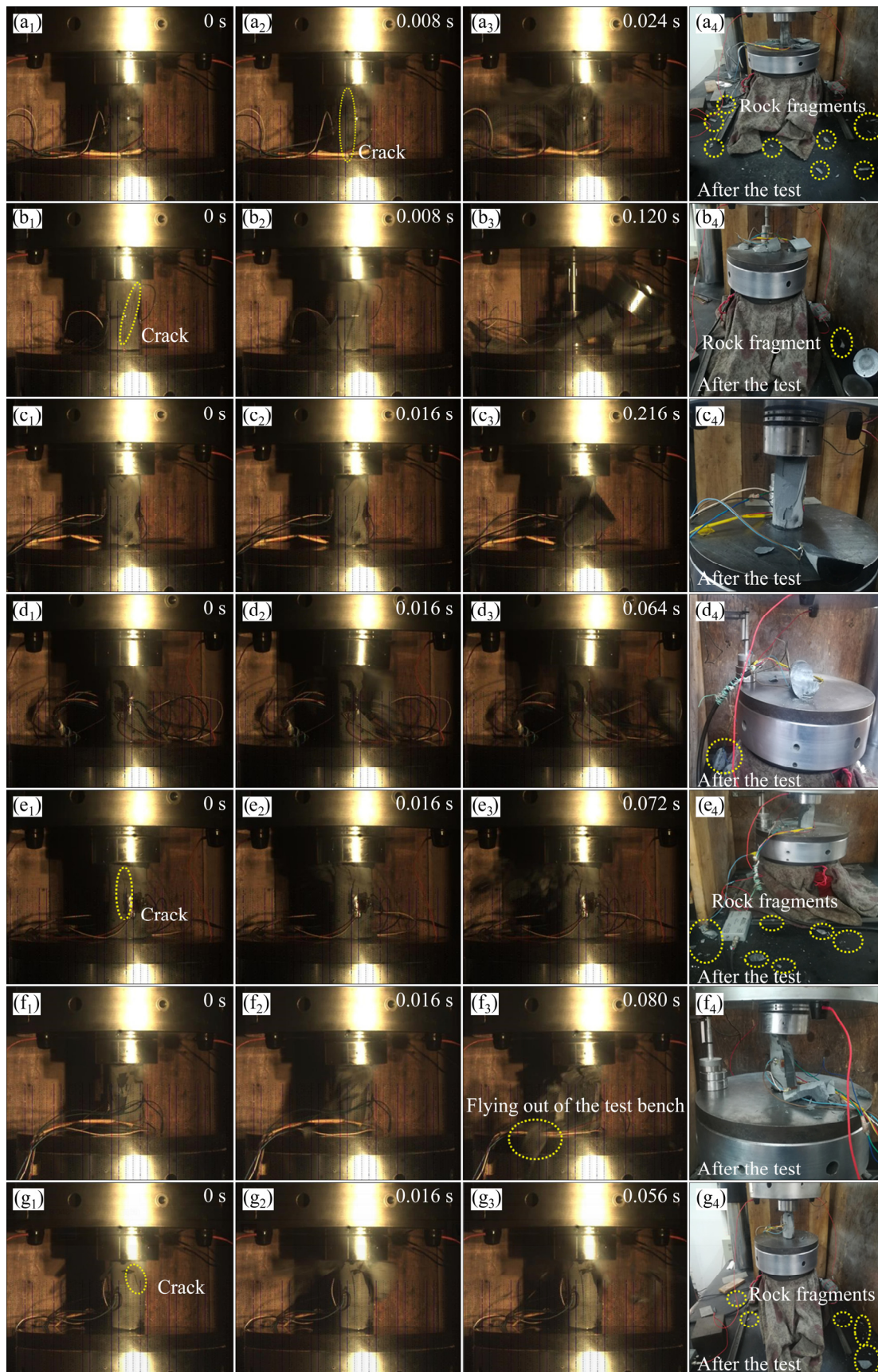
Fig. 14 Failure processes of typical phyllite specimens under different bedding angles: (a) \beta=0^\circ (Specimen 0-1); (b) \beta=15^\circ (Specimen 15-1); (c) \beta=30^\circ (Specimen 30-2); (d) \beta=45^\circ (Specimen 45-1); (e) \beta=60^\circ (Specimen 60-3); (f) \beta=75^\circ (Specimen 75-1); (g) \beta=90^\circ (Specimen 90-2)
