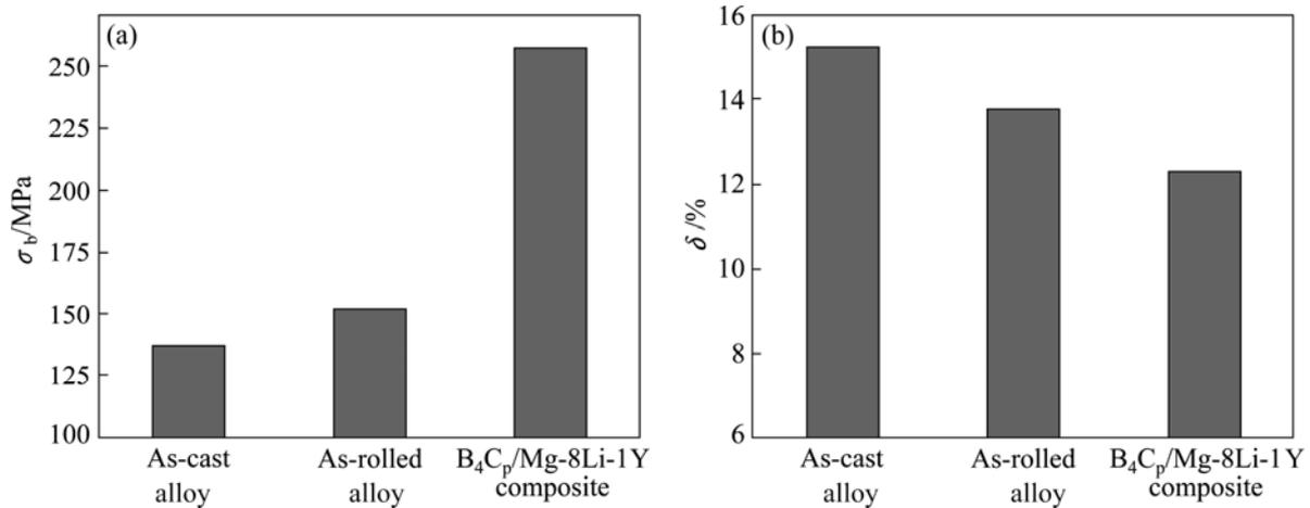
Fig.4 Strength (a) and elongation (b) of Mg-8Li-1Al-1Y alloys
