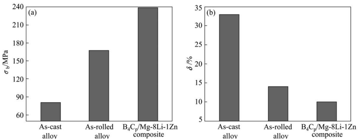
**Fig.3** Strength (a) and elongation (b) of Mg-8Li-1Zn alloys
