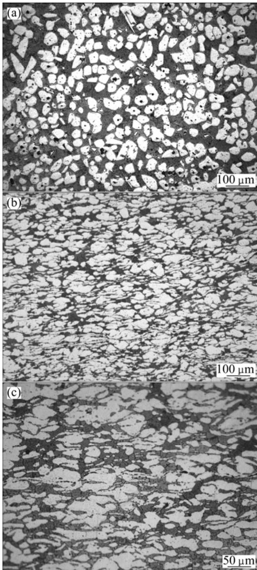
**Fig.2** Microstructures of Mg-8Li-1Al-1Y alloys: (a) As-cast; (b)  $B_4C_p$ /Mg-8Li-1Al-1Y composite (low magnification); (c)  $B_4C_p$ /Mg-8Li-1Al-1Y composite (high magnification)
