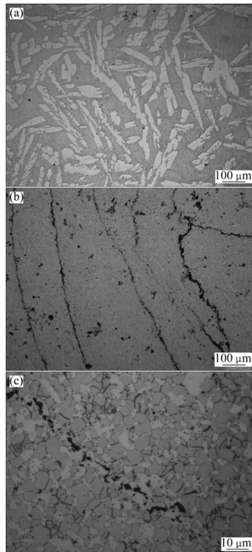
**Fig.1** Microstructures of Mg-8Li-1Zn alloys: (a) As-cast; (b) B<sub>4</sub>C<sub>p</sub>/Mg-8Li-1Zn composite (low magnification); (c) B<sub>4</sub>C<sub>p</sub>/Mg-8Li-1Zn composite (high magnification)
