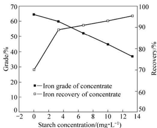
Fig.7 Influence of starch concentration on separation of artificially mixed sample
