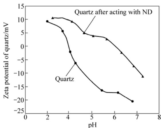
**Fig.9** Zeta potential of quartz before and after acting with ND
