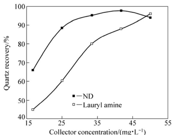
**Fig.1** Influence of collector concentration on floatability of quartz
