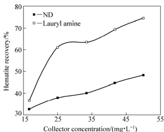
**Fig.2** Influence of collector concentration on floatability of hematite
