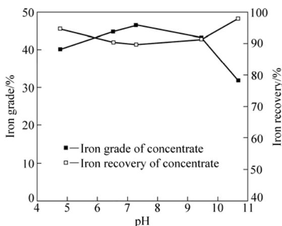
Fig.6 Influence of pH on separation results of artificially mixed sample
