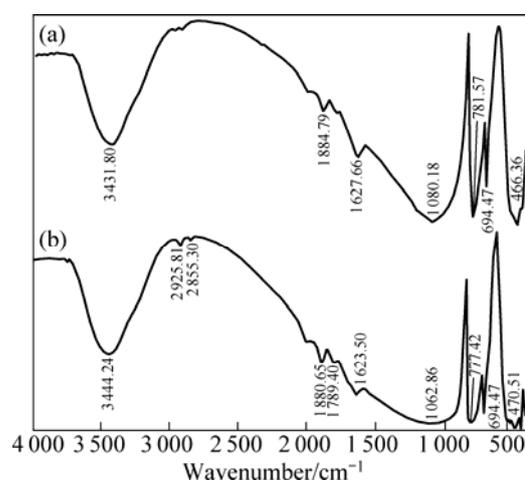
**Fig.10** Infrared spectra of quartz before (a) and after (b) acting with ND
