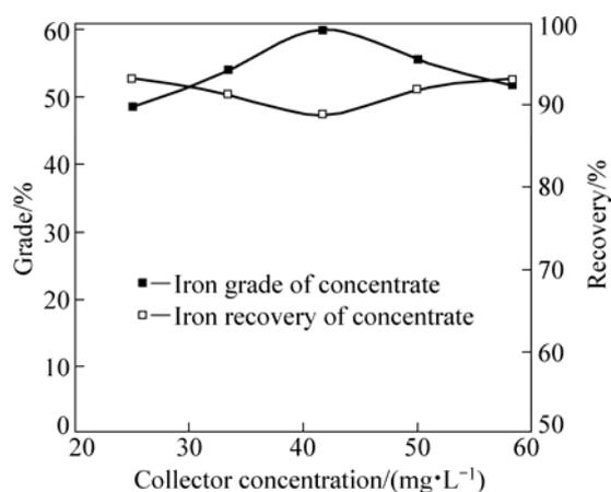
Fig.8 Influence of collector concentration on separation of artificially mixed sample
