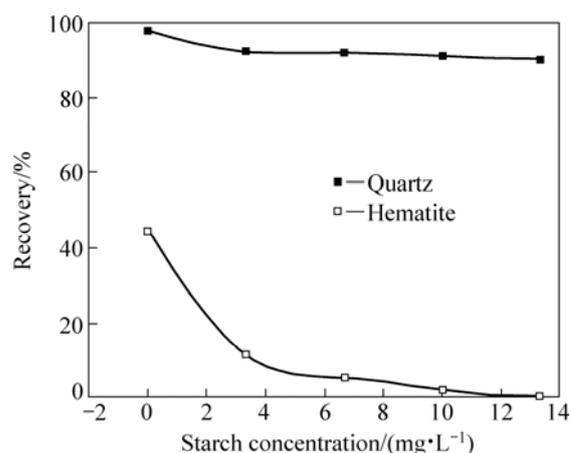
Fig.5 Influence of starch concentration on flotation performances of minerals
