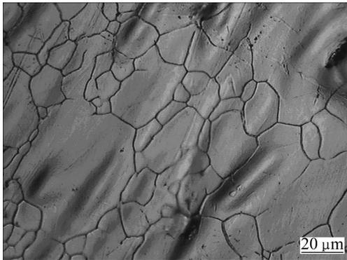
Fig. 2 Microstructure of AZ31 magnesium alloy
