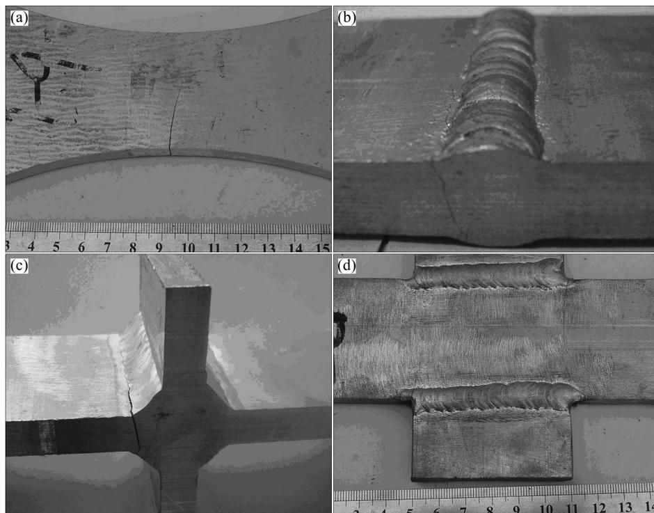
Fig. 5 Fatigue crack initiation, propagation site and direction: (a) Base metal; (b) Butt joint; (c) Transverse cross joint; (d) Lateral connection joint
