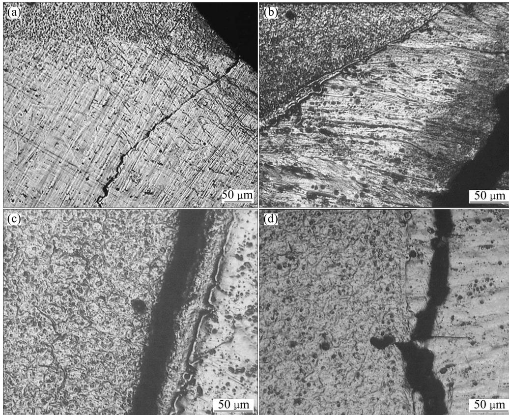
**Fig. 8** Crack propagation site and path for welded joint: (a) Crack propagation site along weld toe; (b) Crack propagation along HAZ; (c), (d) Crack propagation along weld junction
