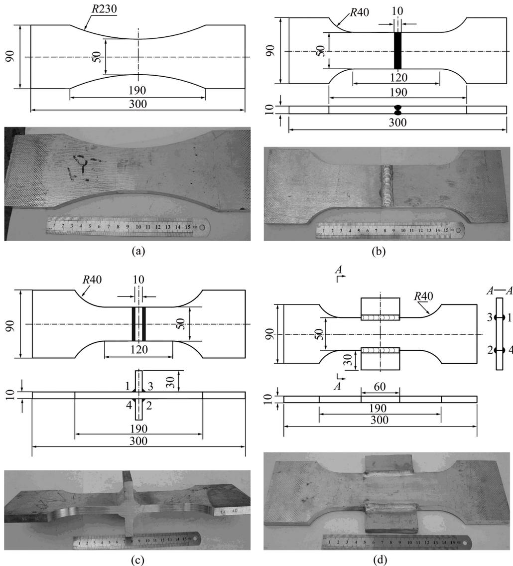
**Fig. 1** Size and shape of AZ31B magnesium alloy fatigue specimens: (a) Base metal; (b) Butt joint; (c) Transverse cross joint; (d) Lateral connection joint (unit: mm)
