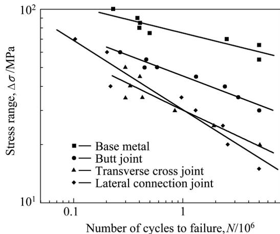
Fig. 4  $S-N$  curves of magnesium alloy AZ31B and welded joints
