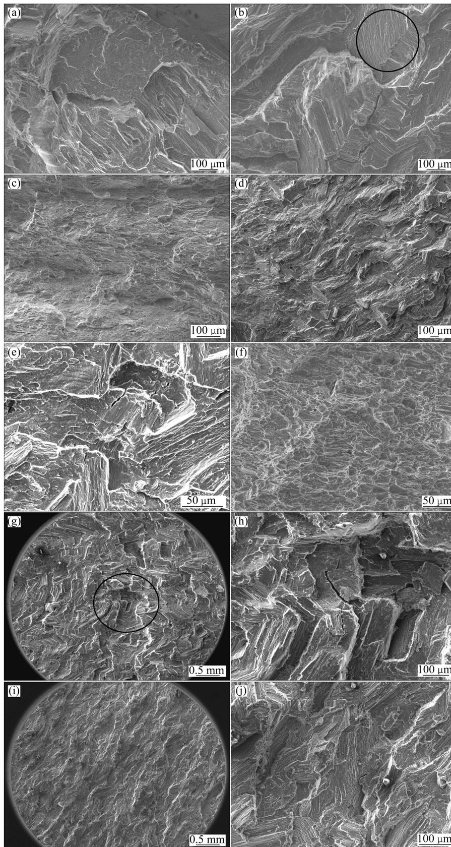
**Fig. 9** Fatigue fracture appearance: (a) Tear ridge on fatigue fracture surface of base metal; (b) Secondary cracks in base metal; (c) Tensile fracture of base metal; (d) Fracture surface of butt joint; (e) Secondary cracks in butt joint; (f) Tensile fracture surface of butt joint; (g) Fracture surface of transverse cross joint; (h) Partial enlargement for Fig. 9(g); (i) Fracture surface of lateral connection joint; (j) Partial enlargement for Fig. 9(i)
