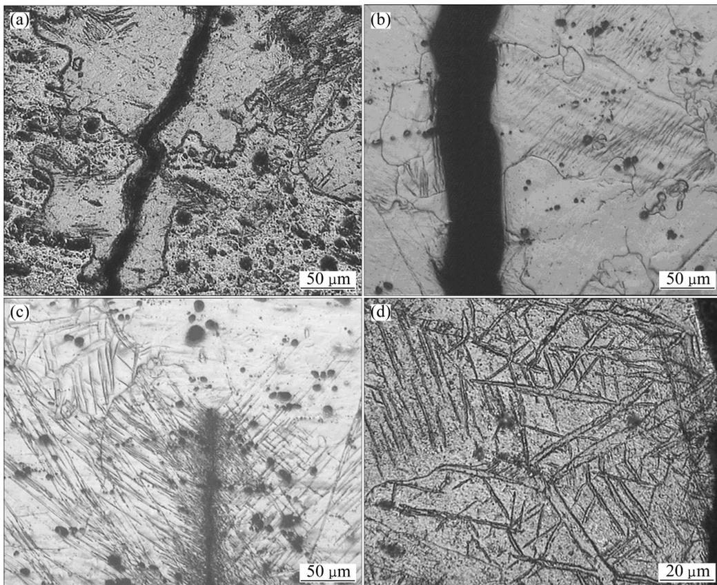
**Fig. 7** Crack propagation path and twinning deformation of base metal: (a), (b) Crack propagation path; (c) Crack tip; (d) Twinning deformation near fracture
