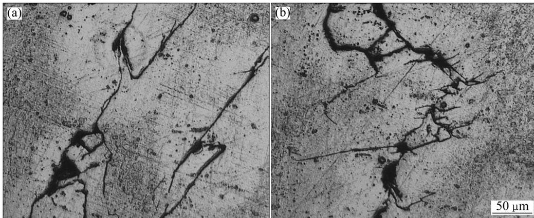
**Fig. 6** Crack propagation path for AZ31B magnesium alloy: (a) Crack branching; (b) Crack propagation path
