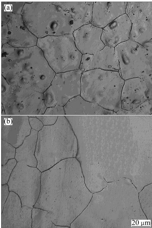
Fig. 3 Microstructures of welded joint: (a) Welding center; (b) HAZ
