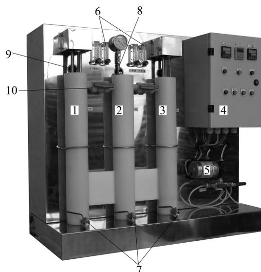
**Fig. 1** Structure of MBR: 1, 2—Reactor column with membrane; 3—Reactor column without membrane; 4—Controller board; 5—Cycle pump; 6—Aeration; 7—Valve of collecting liquid or mineral residue; 8—Position for installing membrane; 9—Position for adding ores; 10—Valve for linking between reactor columns
