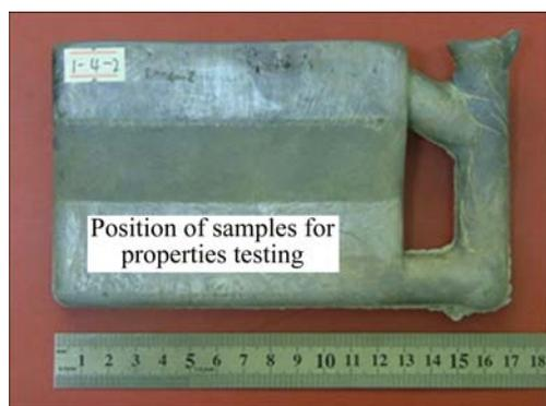
**Fig. 1** Casting with fabricated area of samples for mechanical properties tests
