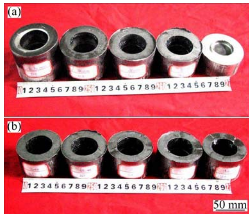
Fig. 11 Extruded cup shells prepared with different billets heights (a) and under different pressures (b)
