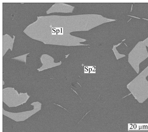
**Fig. 3** Back-scattered electron image of slag oxidized at 1 510  $^\circ\text{C}$  (4% CaO, 4%  $P_2O_5$ ) (Sp1—Rutile; Sp2—Phosphate glassy phase)
