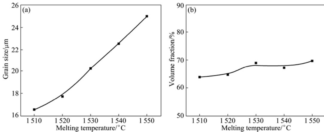
Fig. 4 Relationship between grain size (a) and volume fraction (b) of rutile phase with melting temperature
