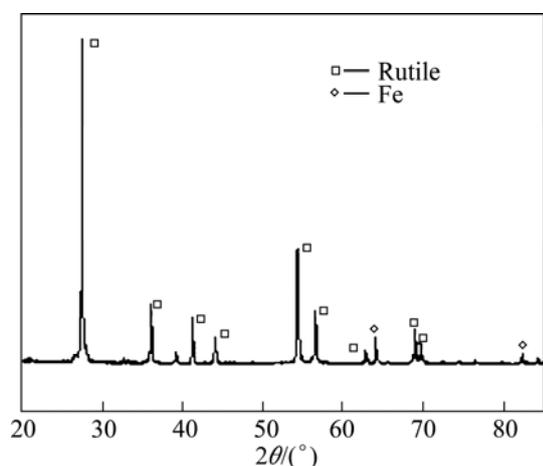
**Fig. 10** XRD pattern of leaching product of modified slag at 1 510 °C
