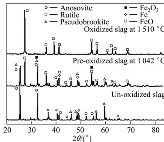
**Fig. 1** XRD patterns of un-oxidized slag and oxidized slag at different temperatures
