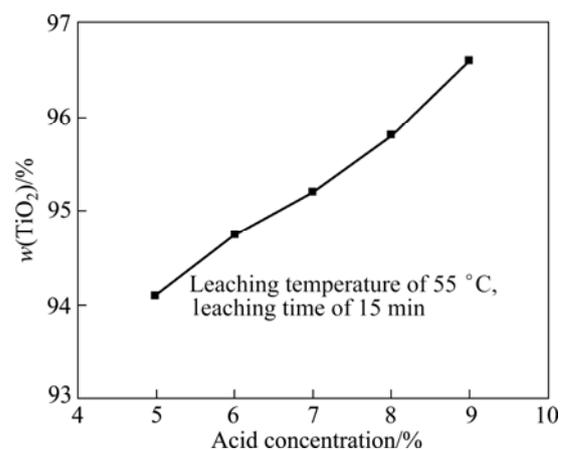
**Fig. 9** Effect of acid concentration on  $\text{TiO}_2$  content in leaching product
