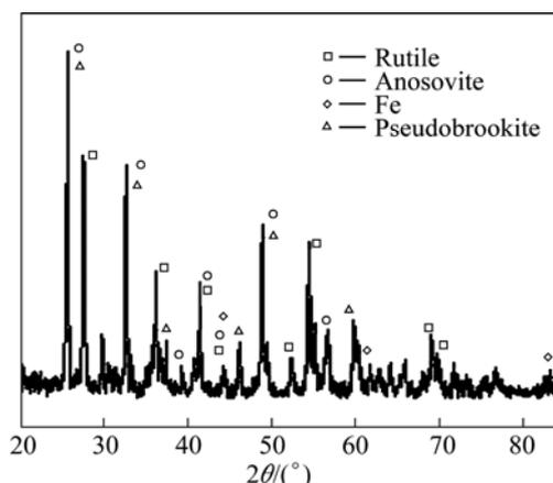
**Fig. 12** XRD pattern of leaching product of slag pre-oxidized at 1 042 °C
