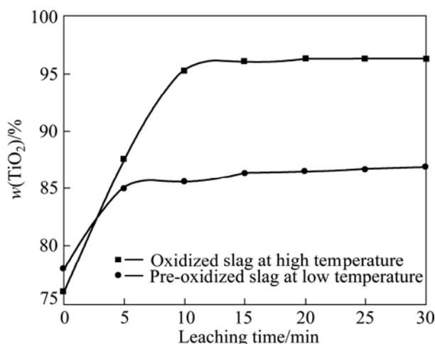
**Fig. 11** Effect of pre-oxidizing at low temperature (around 1 042 °C) and oxidizing at high temperature (1 510 °C) for slag on  $\text{TiO}_2$  content in leaching product (leaching temperature 55 °C, 9% HCl 30 mL, stirring speed 4 r/min)
