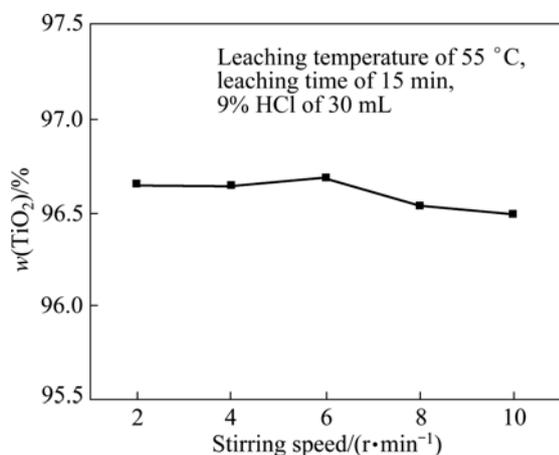
**Fig. 7** Effect of stirring speed on  $\text{TiO}_2$  content in leaching product
