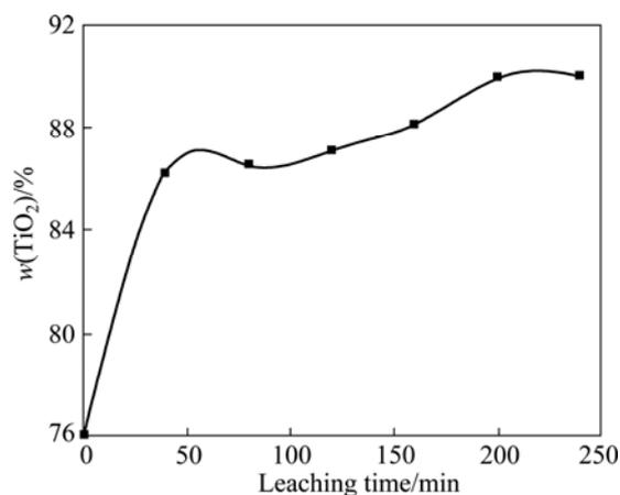
**Fig. 13** Effect of sulfuric acid leaching time on  $\text{TiO}_2$  content in leaching product (leaching temperature 35 °C, stirring speed 4 r/min, 20%  $\text{H}_2\text{SO}_4$  140 mL)
