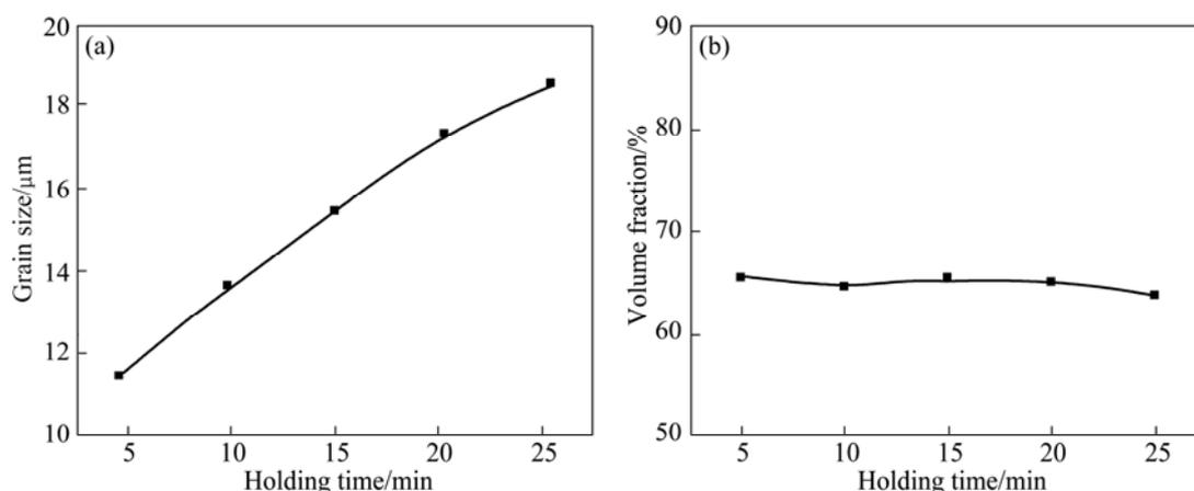
**Fig. 6** Relationship between grain size (a) and volume fraction (b) of rutile phase with holding time
