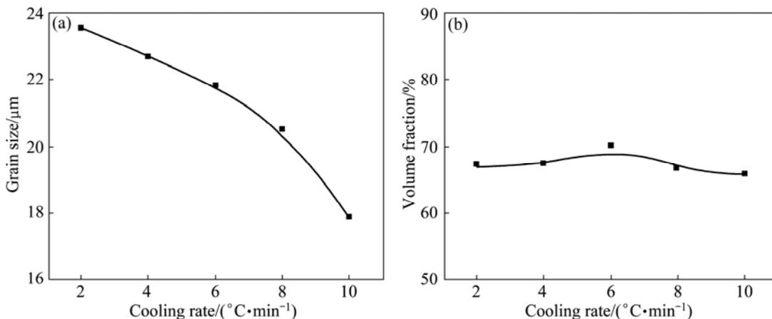
Fig. 5 Relationship between grain size (a) and volume fraction (b) of rutile phase with cooling rate
