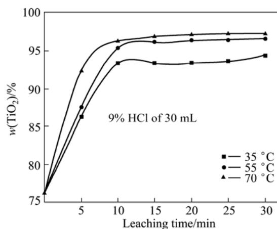
**Fig. 8** Effects of leaching temperature and time on  $\text{TiO}_2$  content in leaching product
