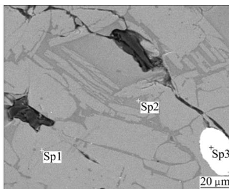
**Fig. 2** Back-scattered electron image of un-oxidized slag (Sp1—Anosovite; Sp2—Silicate glass; Sp3—iron)
