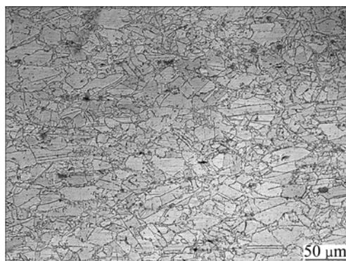
**Fig. 1** Original microstructure of Inconel 718 hot rolling thick plate
