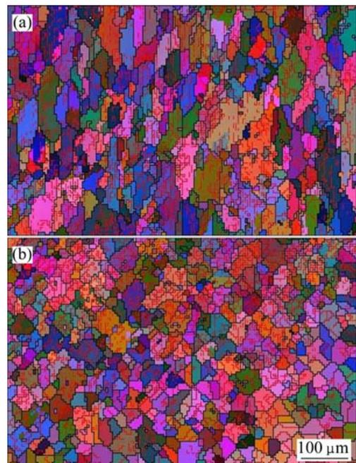
**Fig. 7** Grain map of tube formed at 15.2 MPa in the second corner: (a) Outside; (b) Inside
