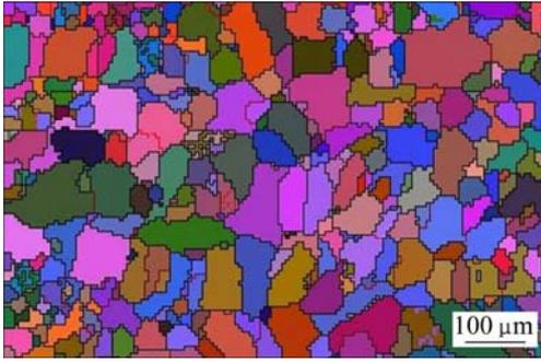
**Fig. 4** Grain map of undeformed annealed tube
