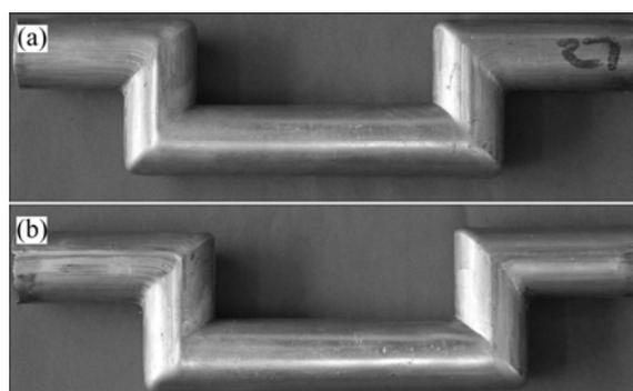
Fig. 2 Shear hydro-bent tube under different internal pressures: (a) 15.2 MPa; (b) 38.0 MPa
