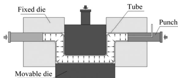
Fig. 1 Principle of shear hydro-bending
