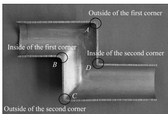
Fig. 3 Schematic diagram of sample: A—Outside of the first corner; B—Inside of the first corner; C—Outside of the second corner; D—Inside of the second corner
