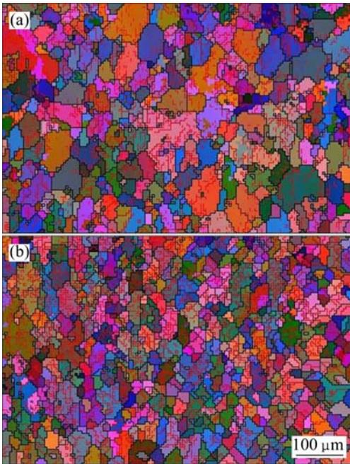
**Fig. 5** Grain map of tube formed at 15.2 MPa in the first corner: (a) Outside; (b) Inside
