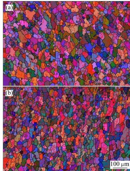
**Fig. 9** Grain map of tube formed at 38.0 MPa in the second corner: (a) Outside; (b) Inside
