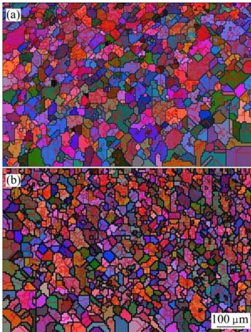
**Fig. 8** Grain map of tube formed at 38.0 MPa in the first corner: (a) Outside; (b) Inside
