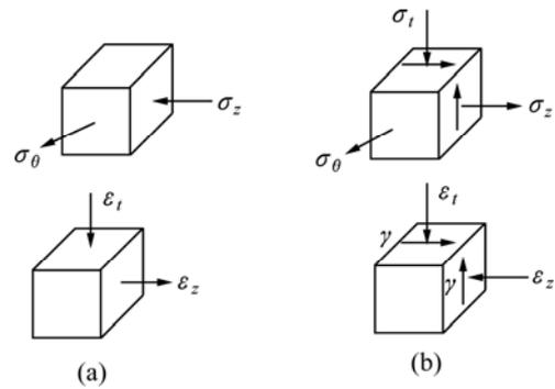
**Fig. 6** Stress and strain of corner zone: (a) Outside corner; (b) Inside corner
