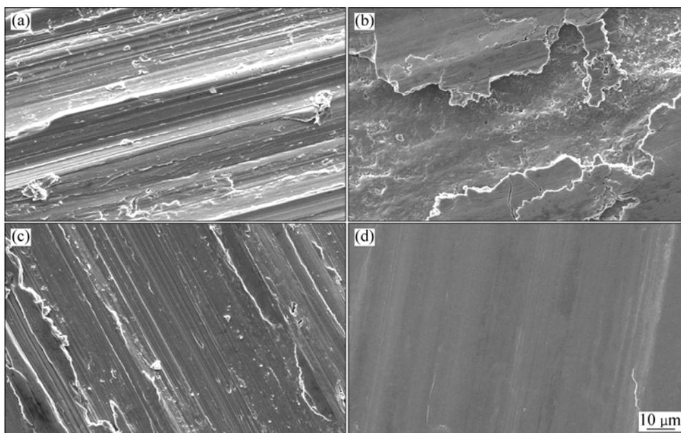
**Fig. 5** Secondary electron images of worn surface of pins tested in air (a) and argon (b) at load of 16 N, and pins tested in air (c) and argon (d) at load of 23 N
