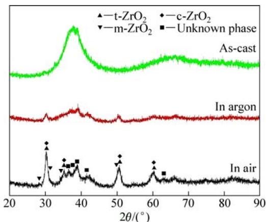
**Fig. 3** XRD patterns of pins before and after wear tests in different environments at load of 23 N
