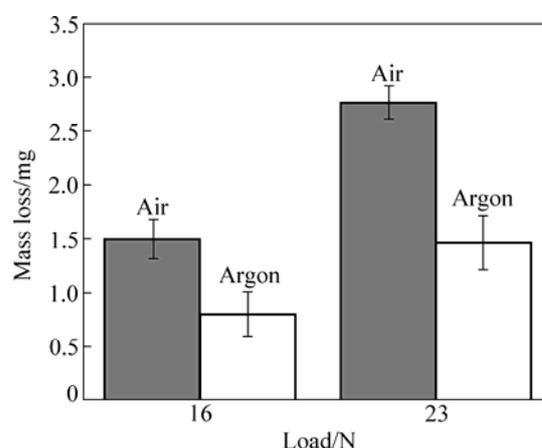
**Fig. 1** Wear loss (mean value of mass loss) of BMG specimens after 1 km-sliding tests in air and argon at different loads (Error bars signify standard deviations)
