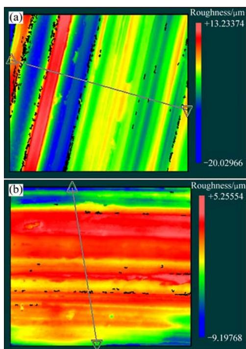
**Fig. 6** Worn surface topographies of pins wear tested in air (a) and argon (b) at load of 23 N determined by optical surface profilometer (Color bands signify the relative height of the profile. Grey lines denote the moving direction of the profilometer)
