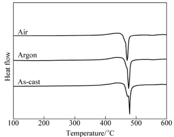
**Fig. 4** DSC curves of pins before and after wear tests in different environments at load of 23 N
