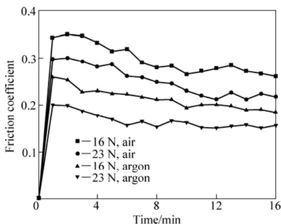
**Fig. 2** Friction coefficients as function of time during wear tests run for 1 km in air and argon under different loads
