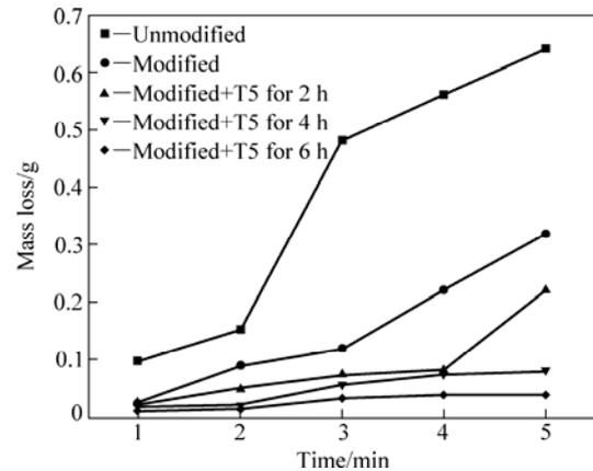
**Fig. 4** Wear resistance of ZL107 Al alloy with or without heat treatment
