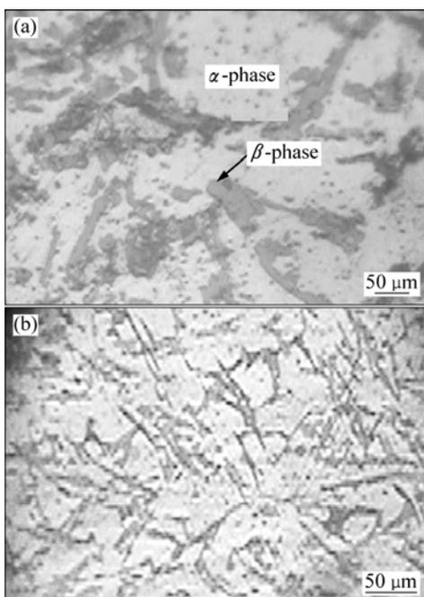
**Fig. 1** Effects of La modification on microstructure evolution of ZL107 alloy: (a) Unmodified; (b) With 1% La modification
