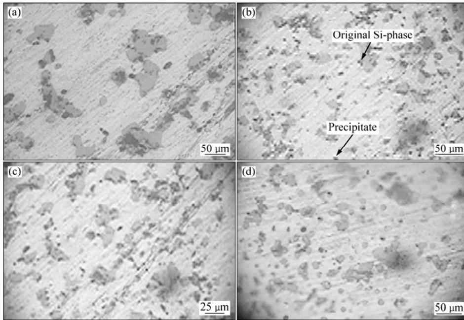
**Fig. 2** Effects of heat treatment on ZL107 alloys: (a) Modification+T4; (b) Modification+T5 for 2 h; (c) Modification+T5 for 4 h; (d) Modification+T5 for 6 h
