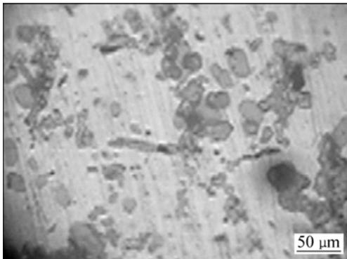
**Fig. 3** Microstructure of unmodified alloys after T5 treatment for 6 h
