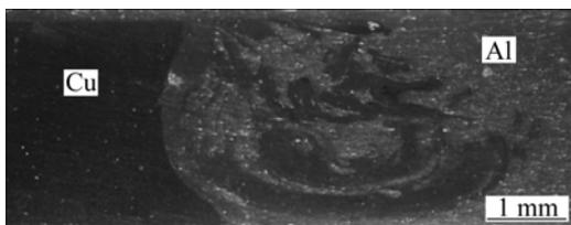
Fig. 3 Optical macrograph showing cross-section structure of dissimilar joint prepared by FSW (Cu lies in AS and Al in RS)
