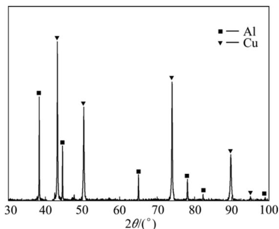
Fig. 6 X-ray diffraction pattern of dissimilar 1350Al-Cu joint
