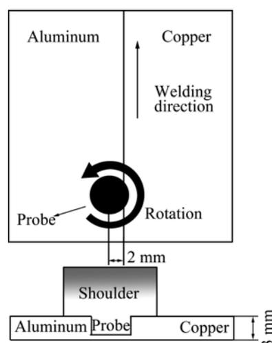
**Fig. 1** Schematic illustration showing set-up of dissimilar FSW
