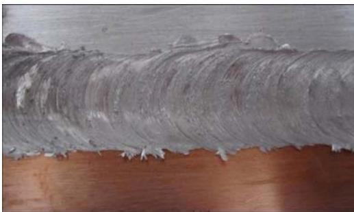
Fig. 2 Surface appearance of dissimilar joint prepared by FSW
