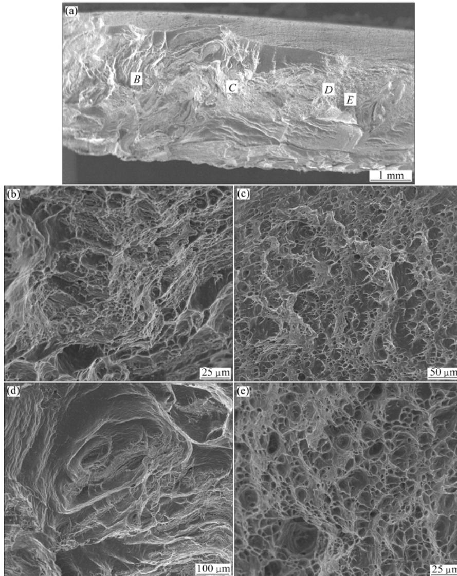
**Fig. 9** SEM images showing tensile fracture surface of Cu–1350Al dissimilar joints:(a) Macrograph of tensile fracture surface; (b)–(e) Magnified microstructures of different regions marked B–E in Fig. 9(a)
