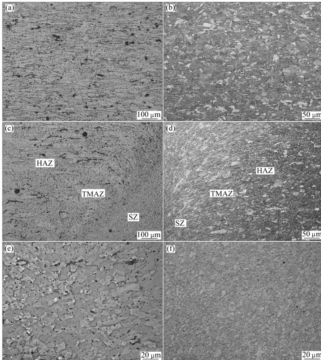
**Fig. 4** Optical microstructures of dissimilar joint in different regions: (a) BM in Al side; (b) BM in Cu side; (c) HAZ and TMAZ in Al side; (d) HAZ and TMAZ in Cu side; (e) SZ in Al side; (f) SZ in Cu side
