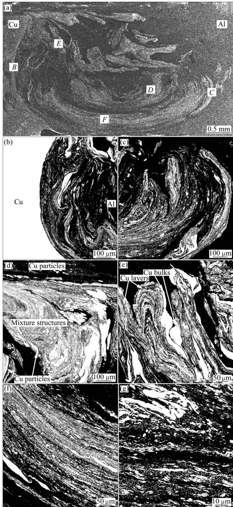
**Fig. 5** SEM images of dissimilar FSW Al-Cu joint: (a) Macrostructure of joint; (b)–(f) BEI images of different regions marked B–F in Fig. 5(a); (g) Magnified view of layer structure as shown in Fig. 5(f)
