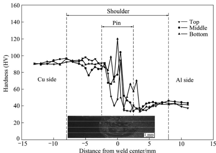
Fig. 7 Hardness profiles measured on cross-section of Cu-1350Al dissimilar weld along top, middle and bottom lines
