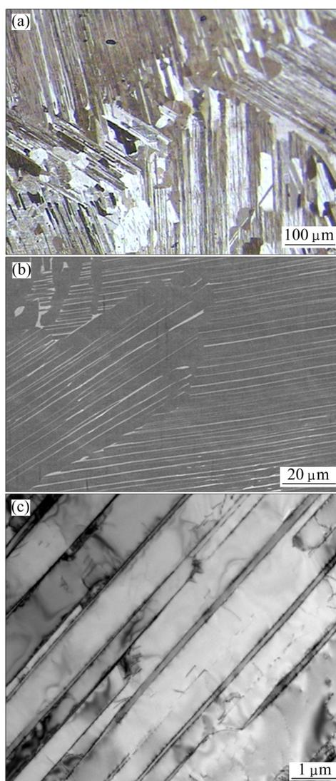
**Fig. 2** Microstructures of TiAl castings: (a) Optical microstructure; (b) SEM image; (c) TEM lamellar microstructure
