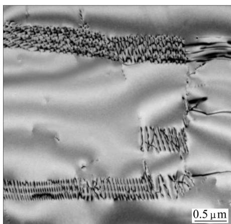
Fig. 6 TEM morphology of dislocations pile-up in slip bands
