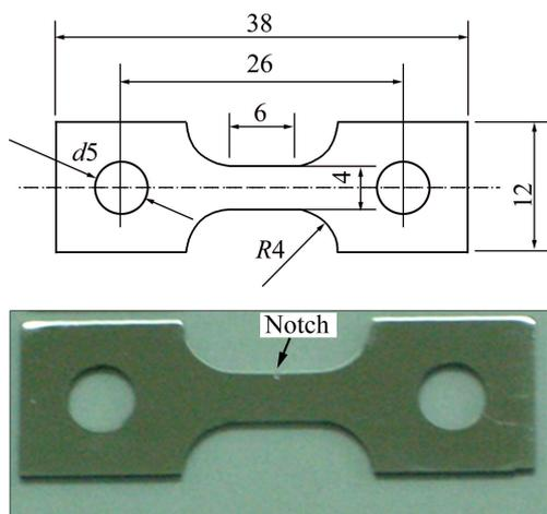
**Fig. 1** Dimensions and macroscopic view of in situ tensile test specimen (Unit: mm)
