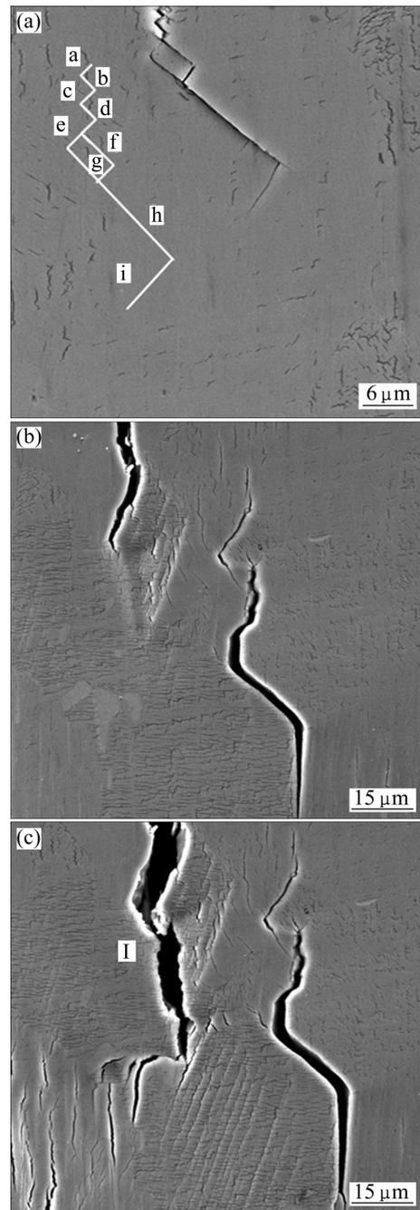
**Fig. 5** SEM images showing initiation and propagation of microcracks in TiAl
