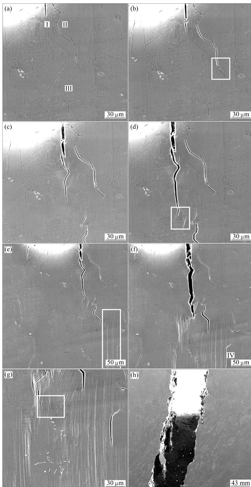
**Fig. 3** Fracture process of TiAl alloy during in-situ tensile test with horizontal loading: (a)–(g) Cracks initiation and propagation under various strains; (h) Failed SEM specimen
