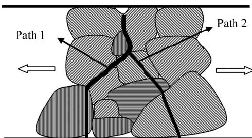
**Fig. 4** Cracks initiation and propagation path of TiAl alloy under in situ tensile test
