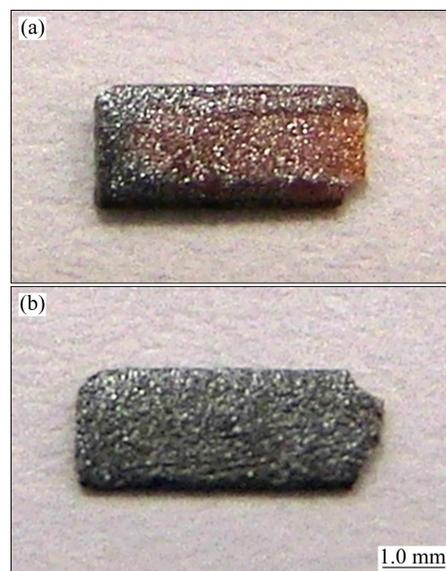
**Fig. 3** Surface morphologies of Ti-Cr alloys after oxidation: (a) Ti-10Cr; (b) Ti-25Cr
