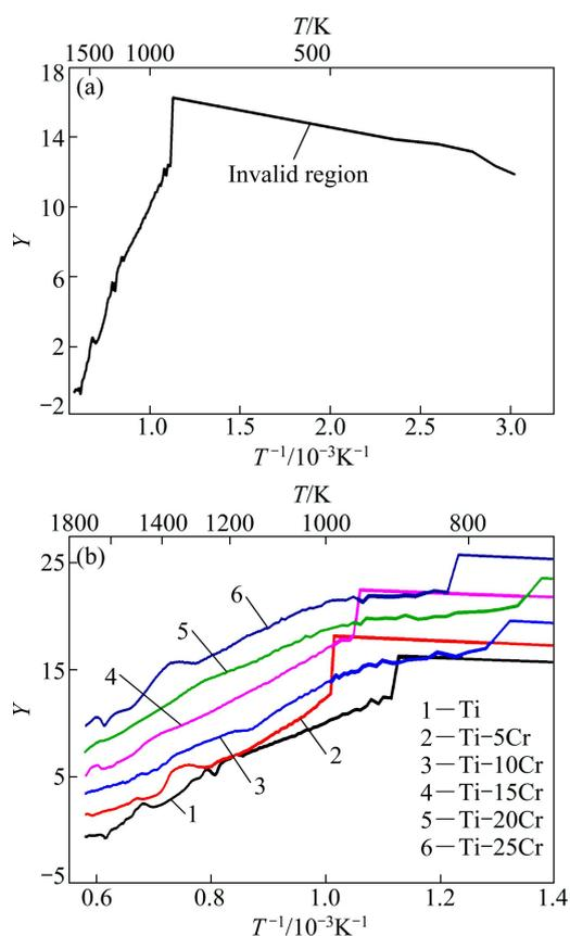
**Fig. 2** Relationship between  $Y$  and  $1000/T$ : (a) Ti, in whole measuring temperature range; (b) At high temperature, to show clearly  $Y$  of Ti-Cr
