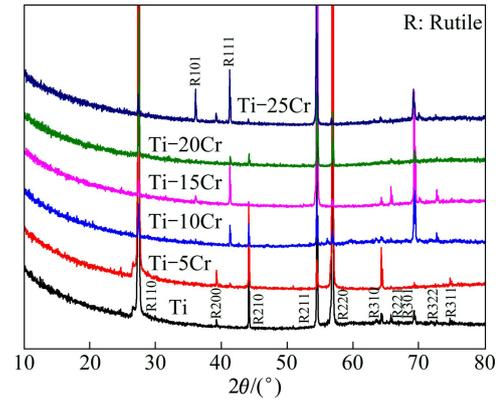
Fig. 4 XRD results of specimen surfaces after oxidation
