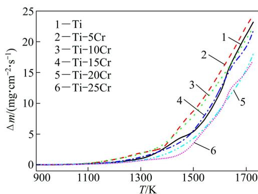
Fig. 1 Mass gain curves of Ti–Cr alloys due to oxidation
