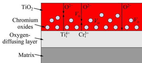
Fig. 6 Microscopic mechanism of oxidation of Ti–Cr alloys
