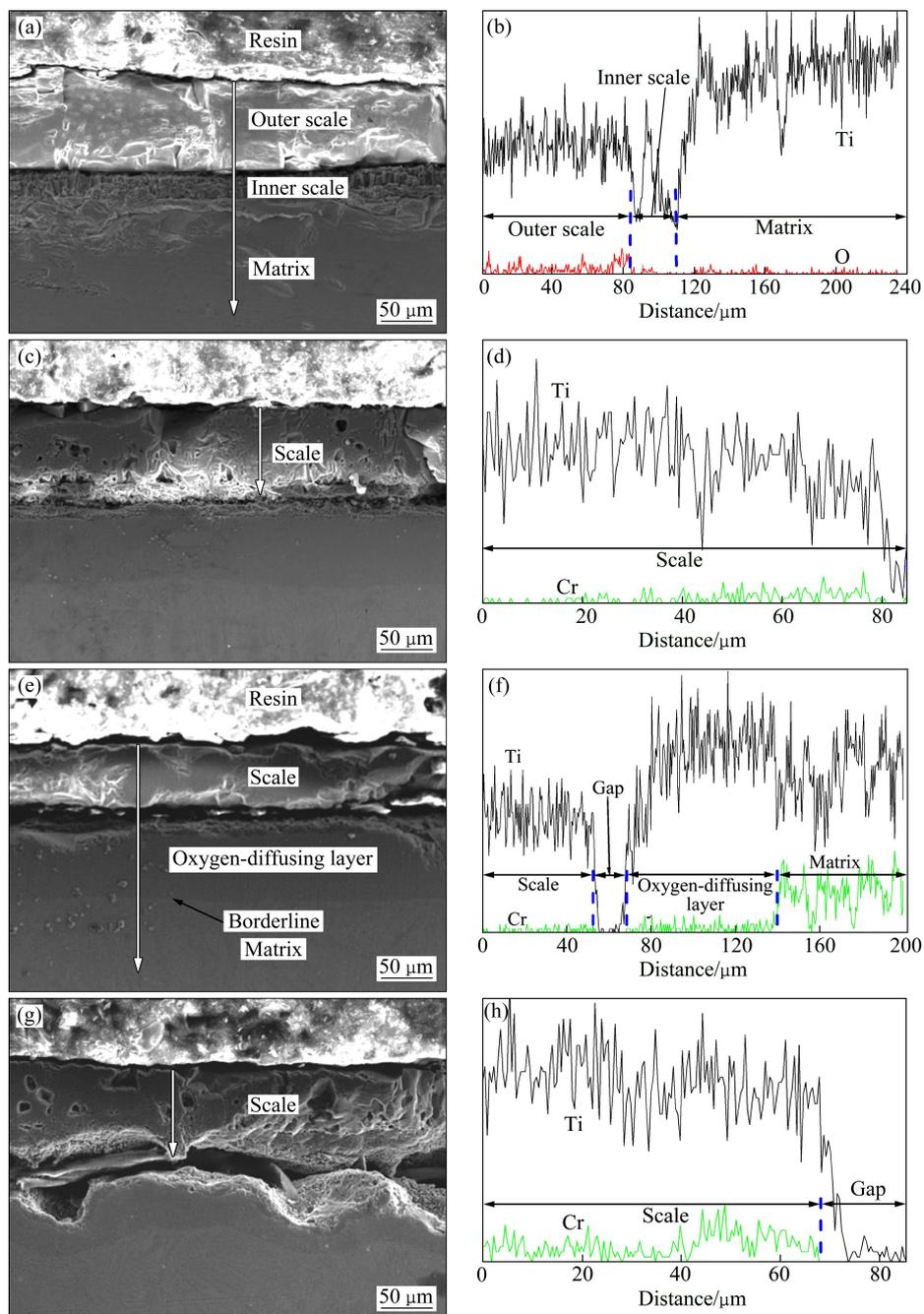
Fig. 5 SEM images and EDS results of Ti–Cr alloys after oxidation: (a), (b) Ti; (c), (d) Ti–15Cr; (e), (f) Ti–20Cr; (g), (h) Ti–25Cr
