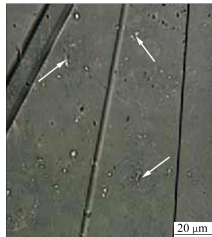
Fig. 4 Precipitates in directionally solidified mc-Si
