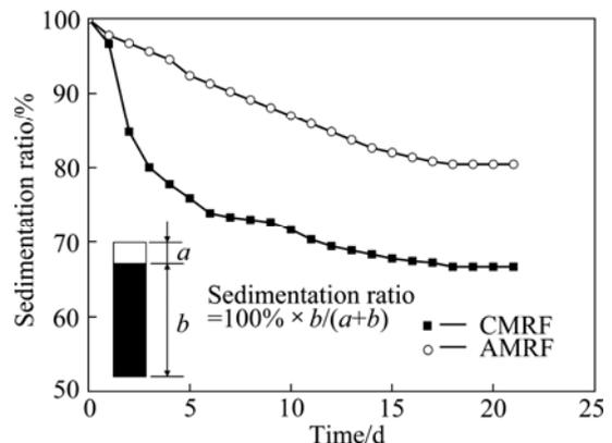
**Fig. 11** Time dependence of sedimentation ratio of CMRF and AMRF
