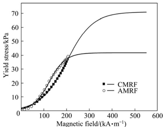
**Fig. 9** Yield stress—magnetic field curves at shear rate of  $200 \text{ s}^{-1}$  for CMRF and AMRF
