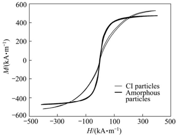
Fig. 5 VSM data of CI particles and amorphous particles
