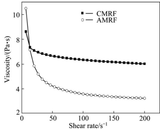
Fig. 7 Viscosity versus shear rate for AMRF and CMRF in the absence of magnetic field
