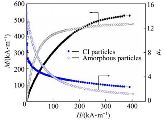
Fig. 6 Dependence of magnetization and permeability on magnetic field of CI particles and amorphous particles
