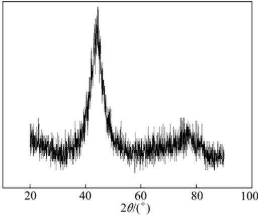
Fig. 4 X-ray diffraction pattern of amorphous particles
