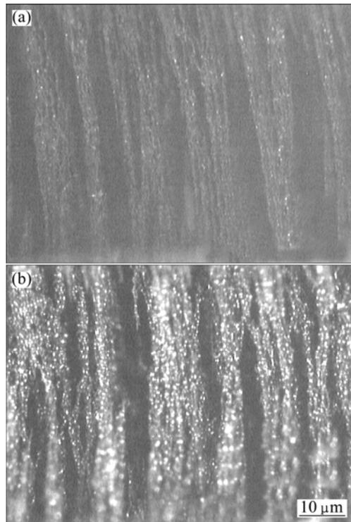
**Fig. 10** Microstructures of CMRF (a) and AMRF (b) at 80 kA/m
