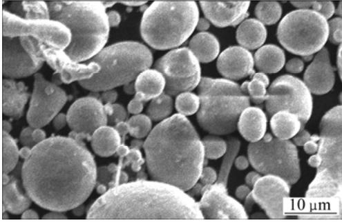
Fig. 3 SEM image of amorphous particles
