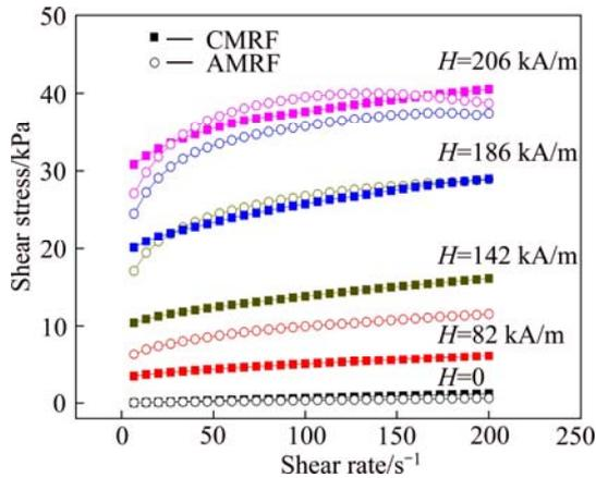
**Fig. 8** Shear stress—shear rate curves for CMRF and AMRF under different magnetic field strengths
