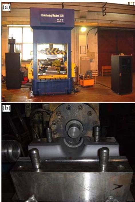
**Fig. 1** Experimental equipment and setup: (a) 3150 kN hydroforming machine; (b) Lower die
