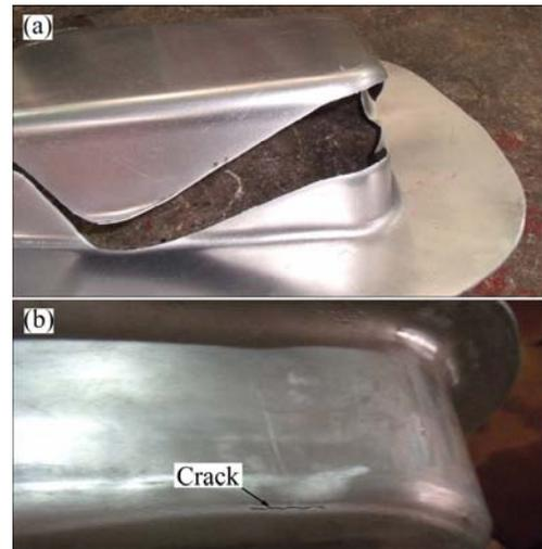
**Fig. 4** Failure types: (a) Fracture at punch nose of corner D; (b) Crack and crease at punch nose near corner B**Table 2** Experiment results with different pre-bulging heights
